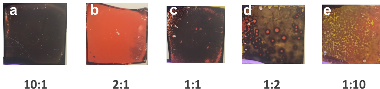
Figure 5.16: Pictures of a mixed perovskites made with melt infiltration
