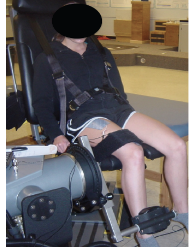
Figure 6: Subject Position for Dynamometer
