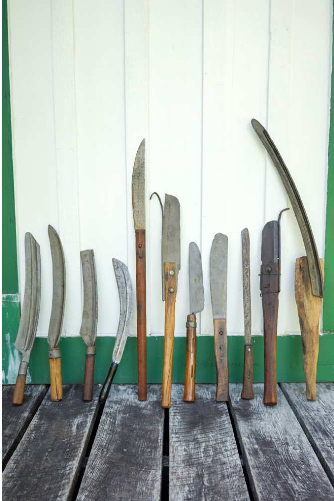
Figure 12. Corn and sorghum cane knives, made from recycled mowing scythes. Of the knife on the far right Jim marvels: “This is just so impractical. I’d hate to be handed that at a corn cutting. I’ve often wondered if it was a joke. I just can’t imagine being that desperate, not being any more creative or having any more skill or talent than to come up with something that crude.” (July 11-a, 2016)
