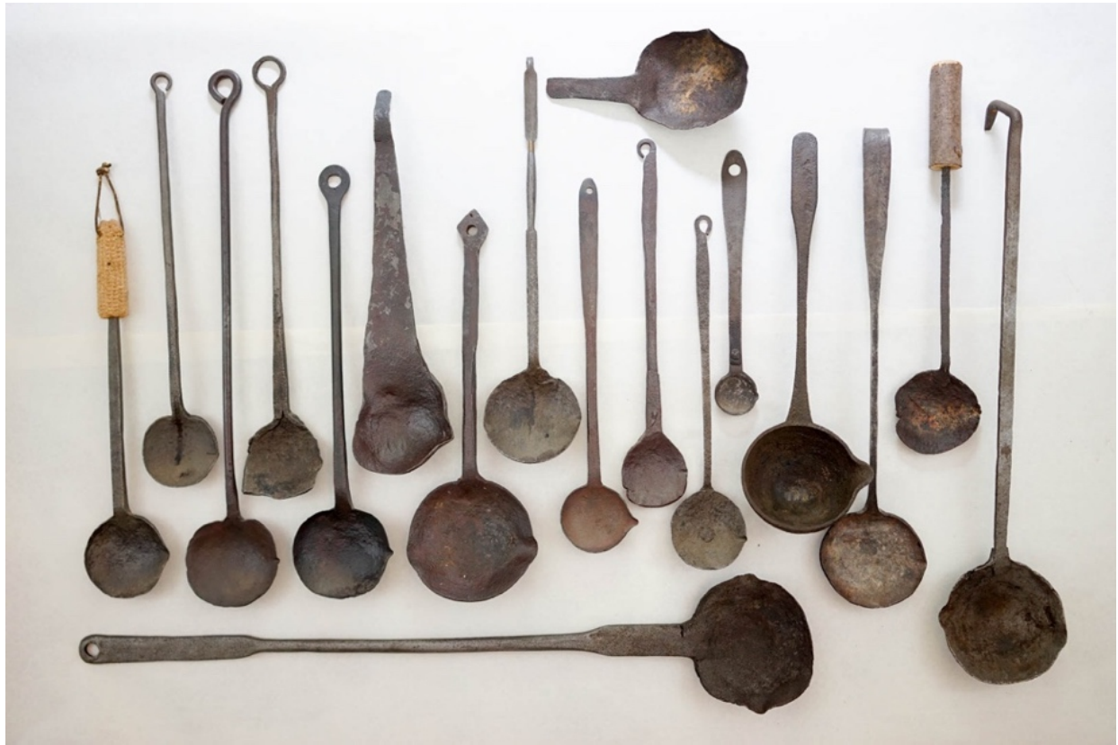
Figure 10. Smelting ladles. Of the sixth ladle from the left, Jim says: "That is the most primitive ladle by far that I own. But it worked, you know? It melted and poured lead just as well as one of these aesthetically pleasing pieces worked. It served the purpose." (June 6-a, 2016)
