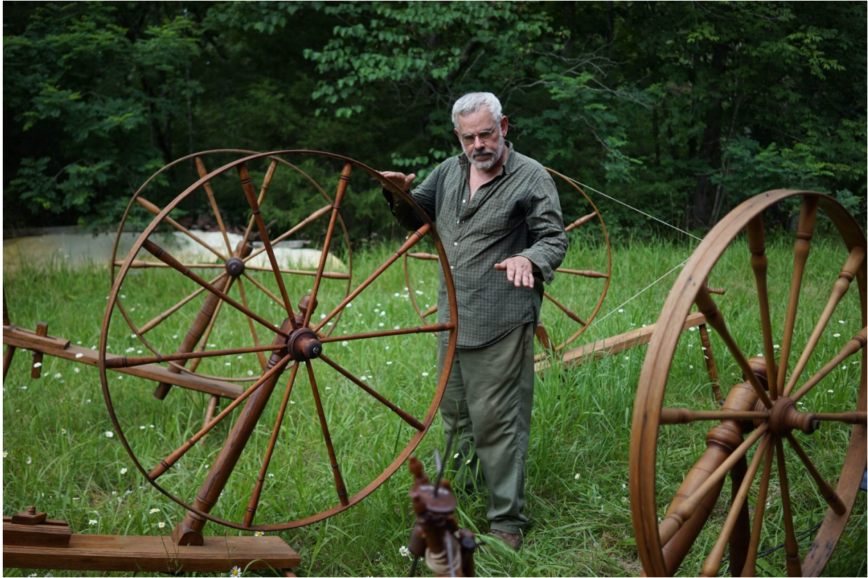
Figure 4. Jim explains the subtle variations in spokes, tensioning devices, and drive wheel posts on his great wheel collection. Some of these personal touches improve function, while others are decorative choices.
