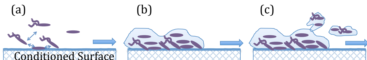
Figure 1.3. Stages of biofilm formation on a membrane surface. Blue arrows represent the direction of water flow. (a) Initial attachment: bacteria sense/adjust to their environment, communicate via chemical signaling, and attach to membrane surface. (b) Biofilm formation: bacteria excrete extracellular polymeric substances (EPS), grow, reproduce and form a complex matrix known as a biofilm. (c) Plateau phase: growth and detachment of bacteria and/or matrix reach equilibrium, with detachment occurring due to shear forces.
