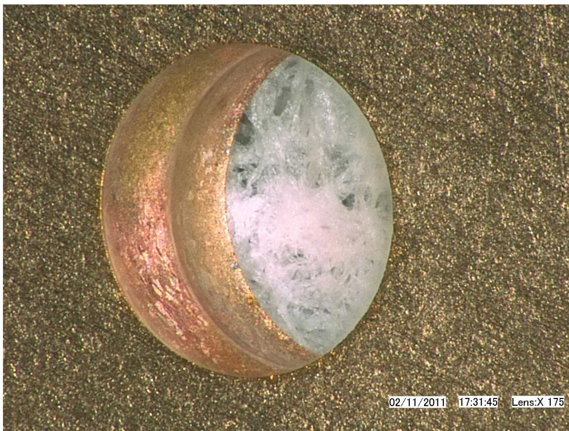
Figure 2.13: Image taken at 30° angle of 1 mm cylindrical ring electrode hole formed by wet chemical etching a piece of copper sheet metal. The cusp feature created by the two sided isotropic chemical etching process is visible inside the hole.
