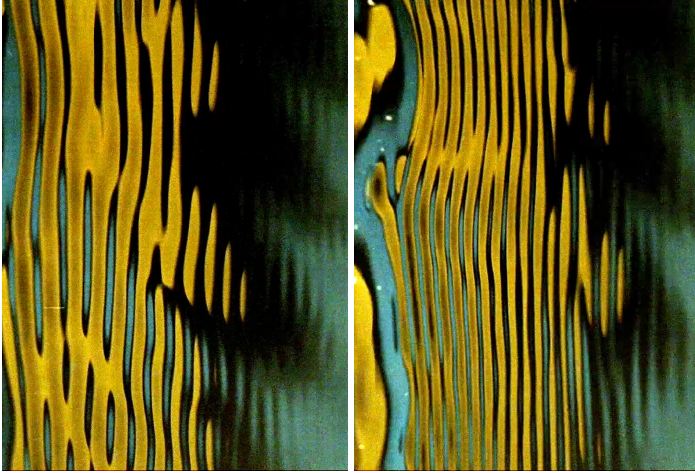
Figure 4.3: Color enhanced images of a fluid surface at two times showing expansion and contraction of capillary waves excited by a cylindrical obstacle placed just below the surface of the fluid, which moved with a constant background flow speed.
