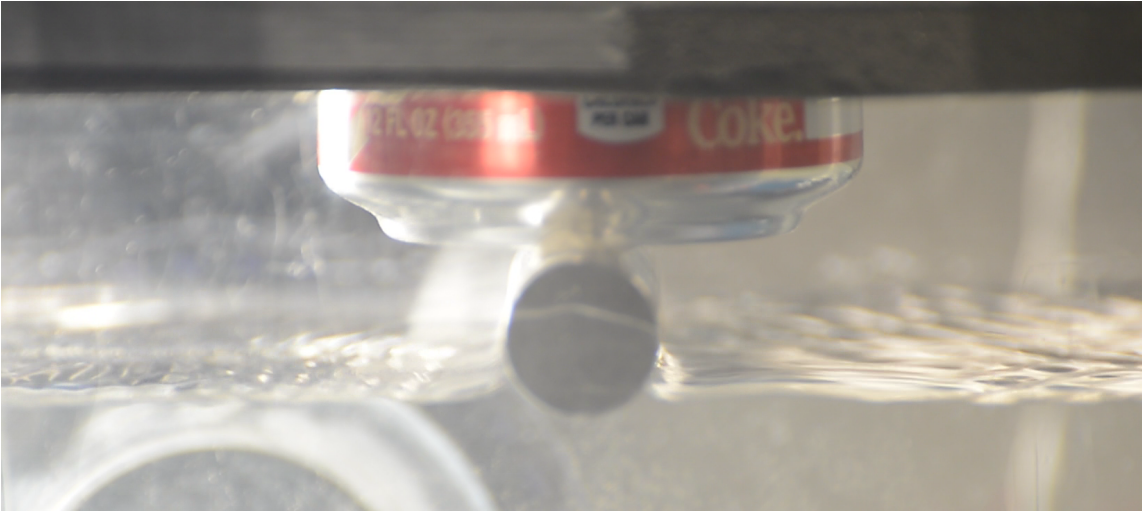
Figure 4.1: The surface of constant background fluid flow is disturbed by a partially submerged cylinder. Relatively short wavelength capillary waves are shown upstream (to the left) of the obstacle. Experimental observations agree well with predictions from linear wave theory.
