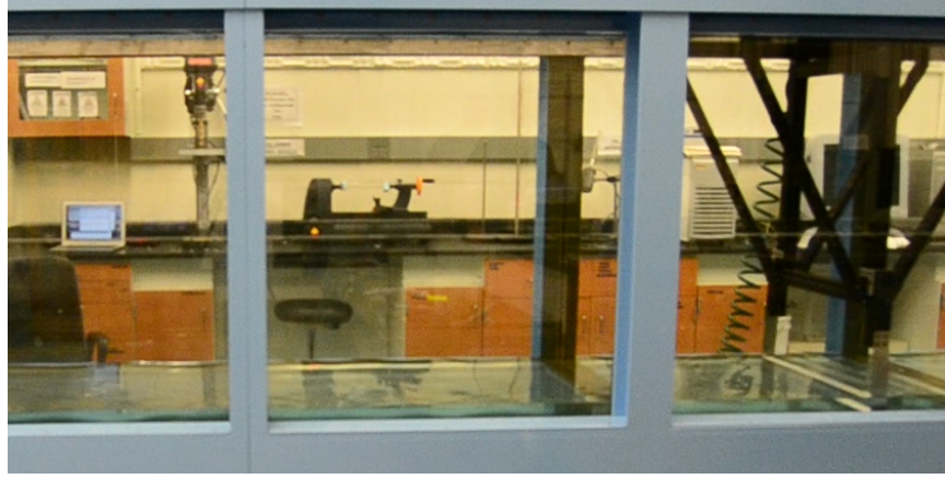
Figure 4.6: A frame of video taken of the experimental setup described in this section. An obstacle 0.6 cm in height and 4.5 cm wide is towed at the bottom of 5.3 cm of water at a rate of 48.61 cm per second. Disturbances in the shape of solitary waves were observed propagating ahead of the obstacle.
