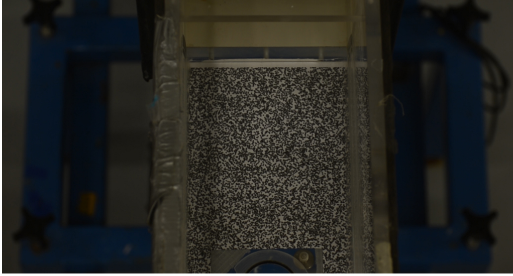
Figure 4.4: Experimental image of a top view of a fluid recirculating flume with water moving from top to bottom in the image and a transparent bottom with a random dot pattern attached below for use with the surface Schlieren technique described in [19].
