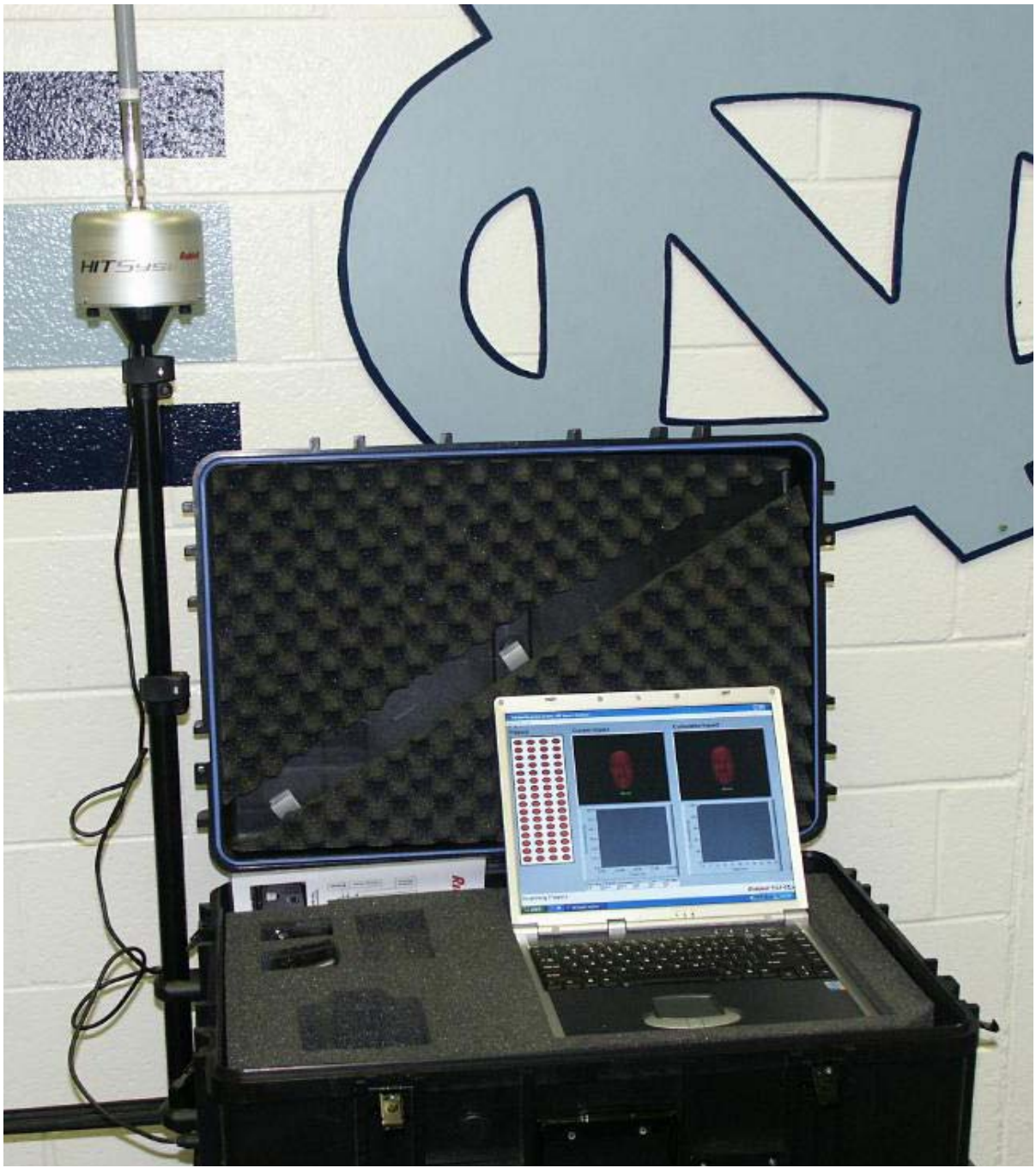
Figure 2. Sideline control unit that stores and displays the information collected.
