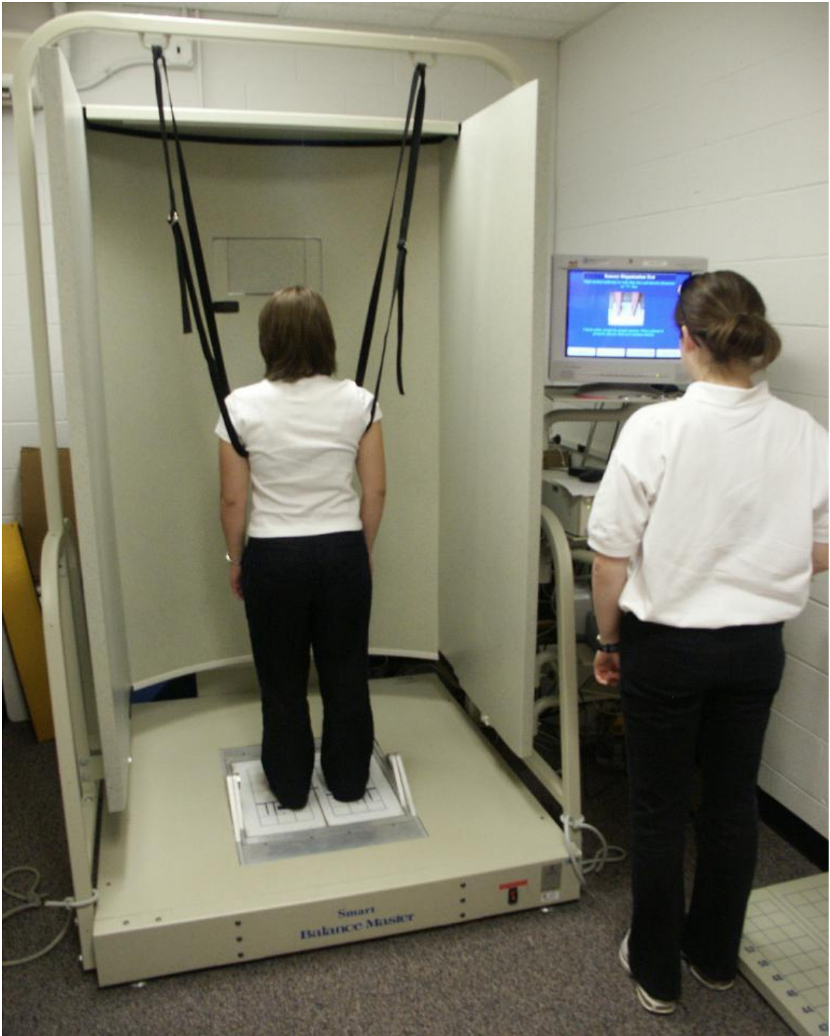
Figure 4. NeuroCom used for the SOT test which assesses balance performance.
