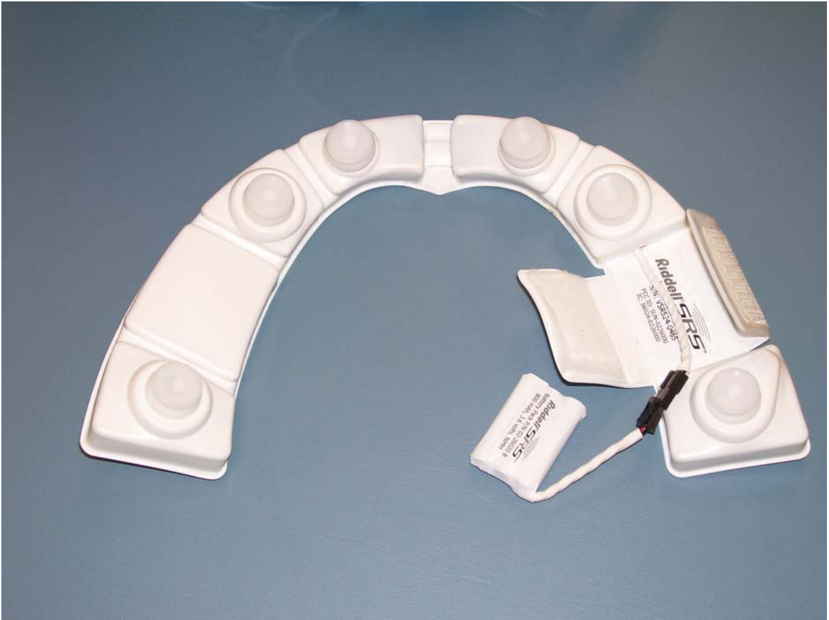
Figure 1. Accelerometers that fit into the Riddell Helmets.
