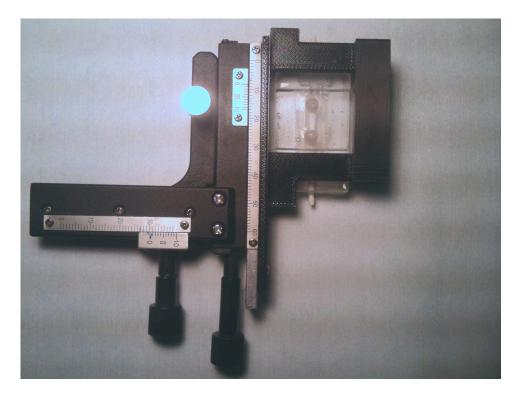
Figure 3.7 Custom built stage to secure the MCA device to the tilting microscope.
