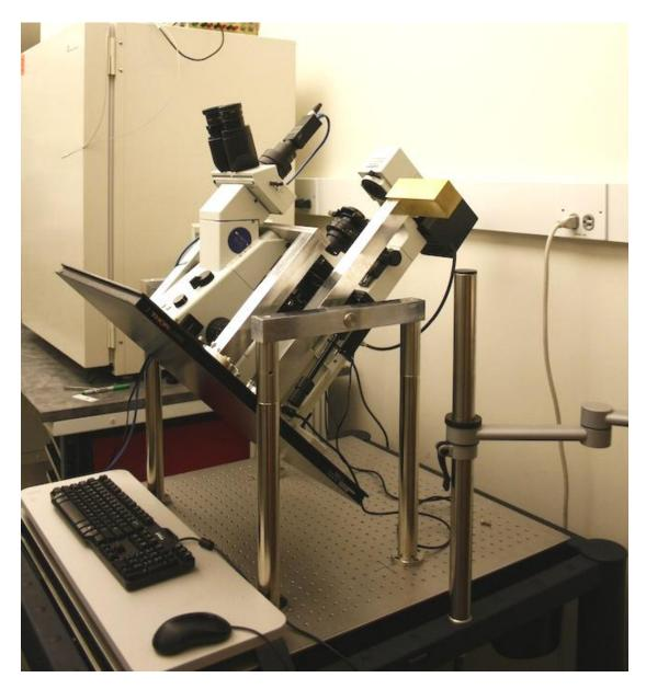
Figure 5. 1 The custom built microscope IXION. The microscope is capable of bright field, phase, and epifluorescense microscopy and can be tilted so that the optical path is 30, 45, 60, or 90 degrees from vertical.
