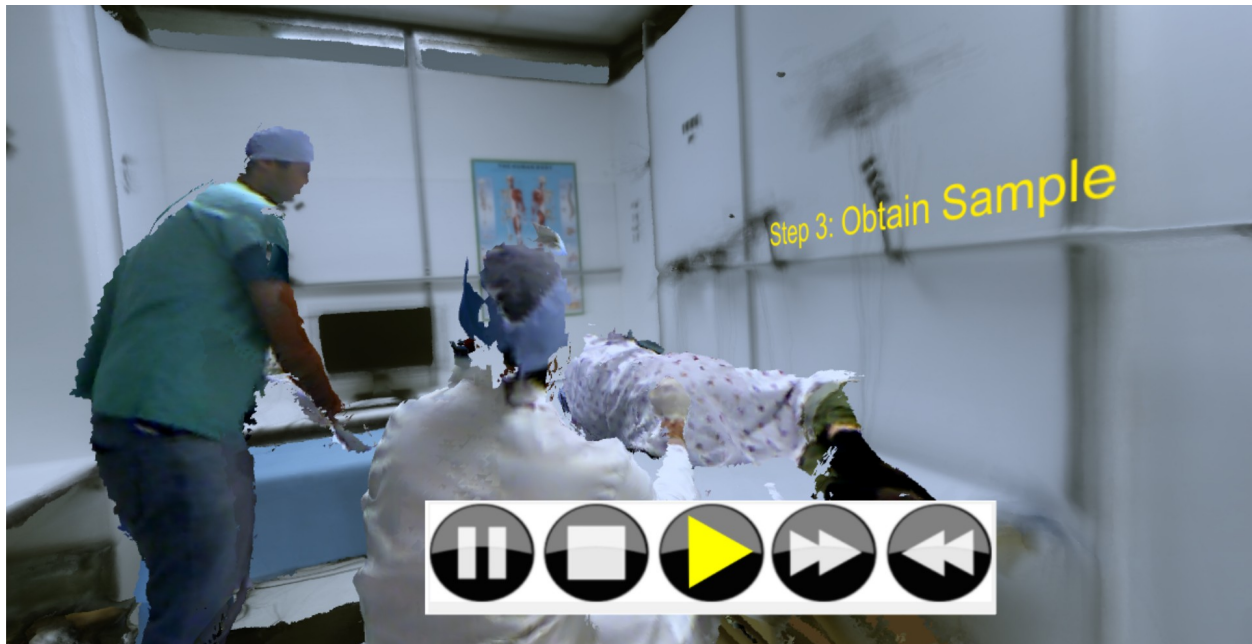
Figure 12: Screenshot of mock procedure playback viewed in an Oculus Rift headset and rendered with the Unity Game Engine. Notice the annotation along the wall in the scene and the playback control panel floating in front of the user's face.
