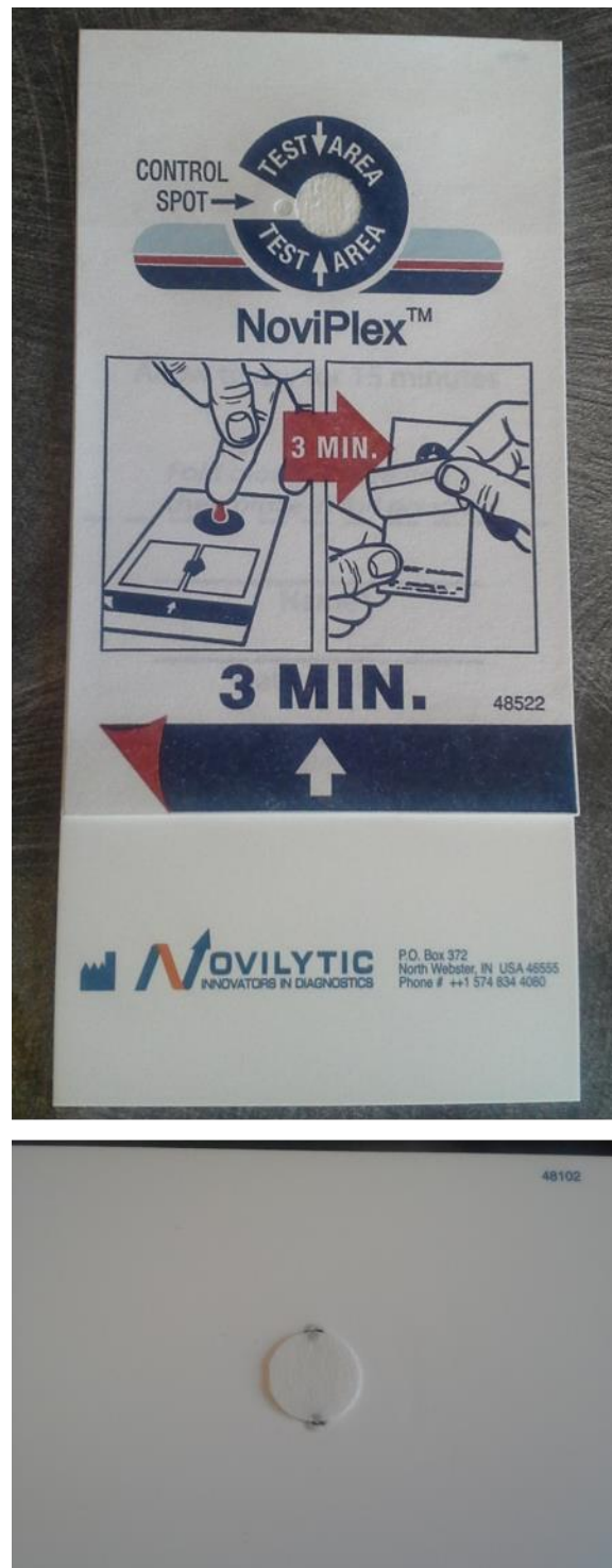
Figure 1.2: Noviplex plasma collection card. Top: The Noviplex card with filter membrane. Bottom: The paper sampling disc with the filter membrane removed.
