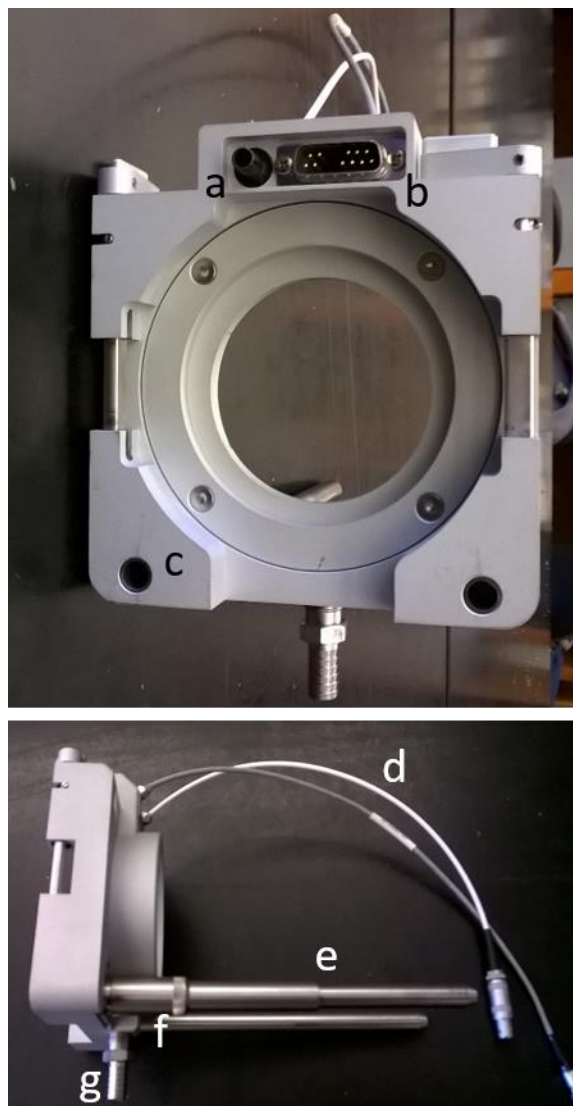
Figure 4.2: The Velox 360 mounting flange. Major parts: a) high voltage connection; b) interlock connection; c) alignment holes; d) high voltage and interlock cables; e) support rods; f) positioning screw; g) vent port.
