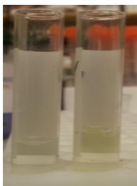
Figure 21: AST-IV activity confirmation. The by-product of the AST-IV reaction is PNP, and has a yellow tint to it when in a clear solution. The solution on the right in the above picture has AST-IV compared to the solution on the left that does not have AST-IV. The yellow tint indicates active AST-IV.
