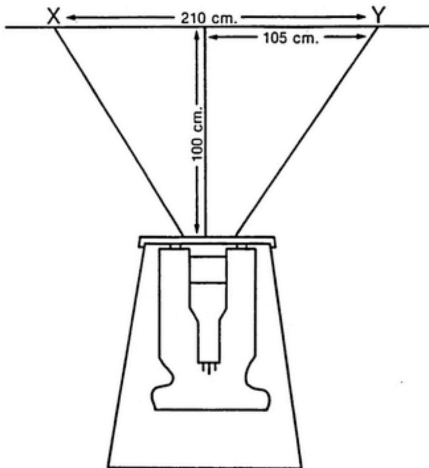
Figure 9. Dimensions of Solid Angle Geometry
