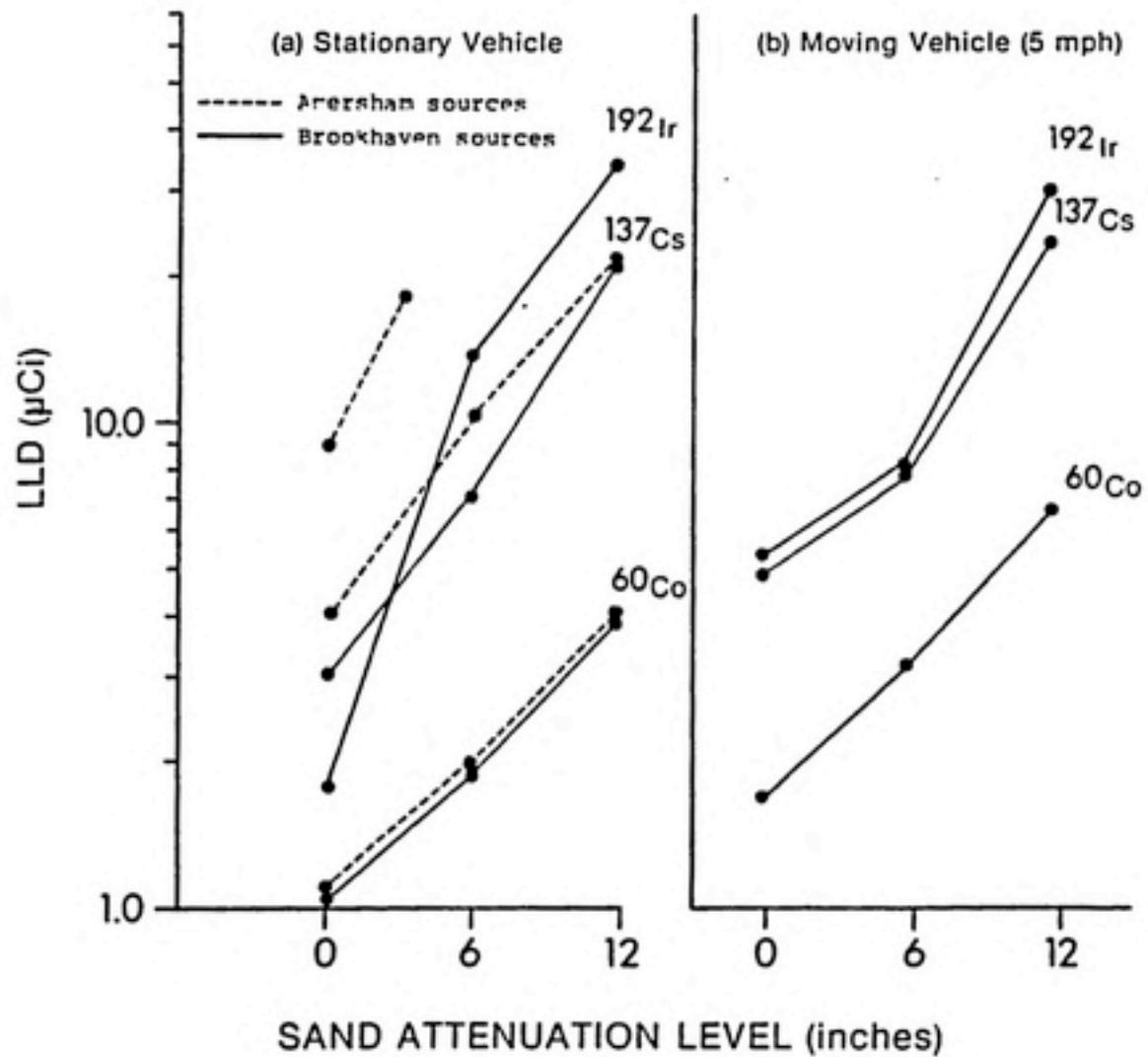
Figure 17. LLD Curves for Brookhaven Sources (Dead Time Corrected Values) on Stationary and Moving Vehicle
