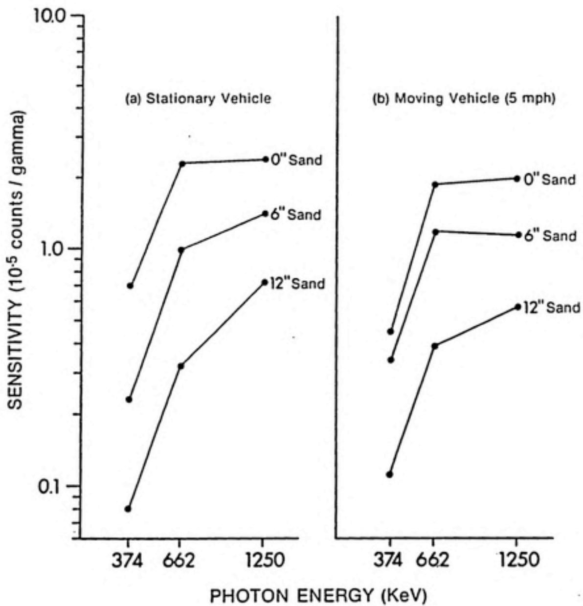
Figure 12. Sensitivity Curves for Stationary and Moving Vehicle, Brookhaven Sources
