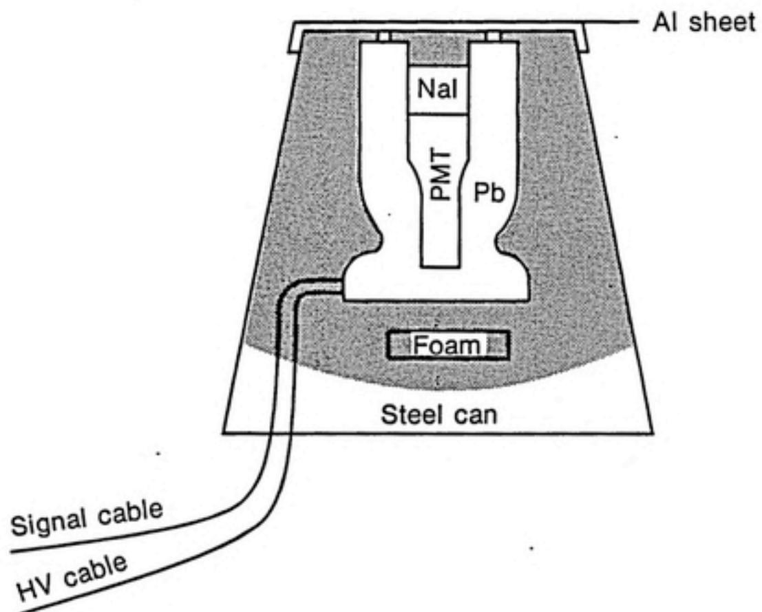
Figure 2. Detector Head Assembly
