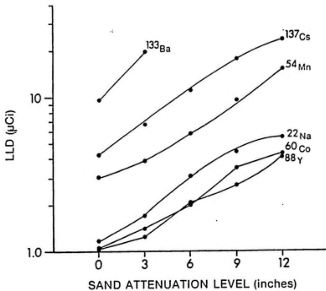
Figure 16. LLD Curves for Amersham Sources on Stationary Vehicle
