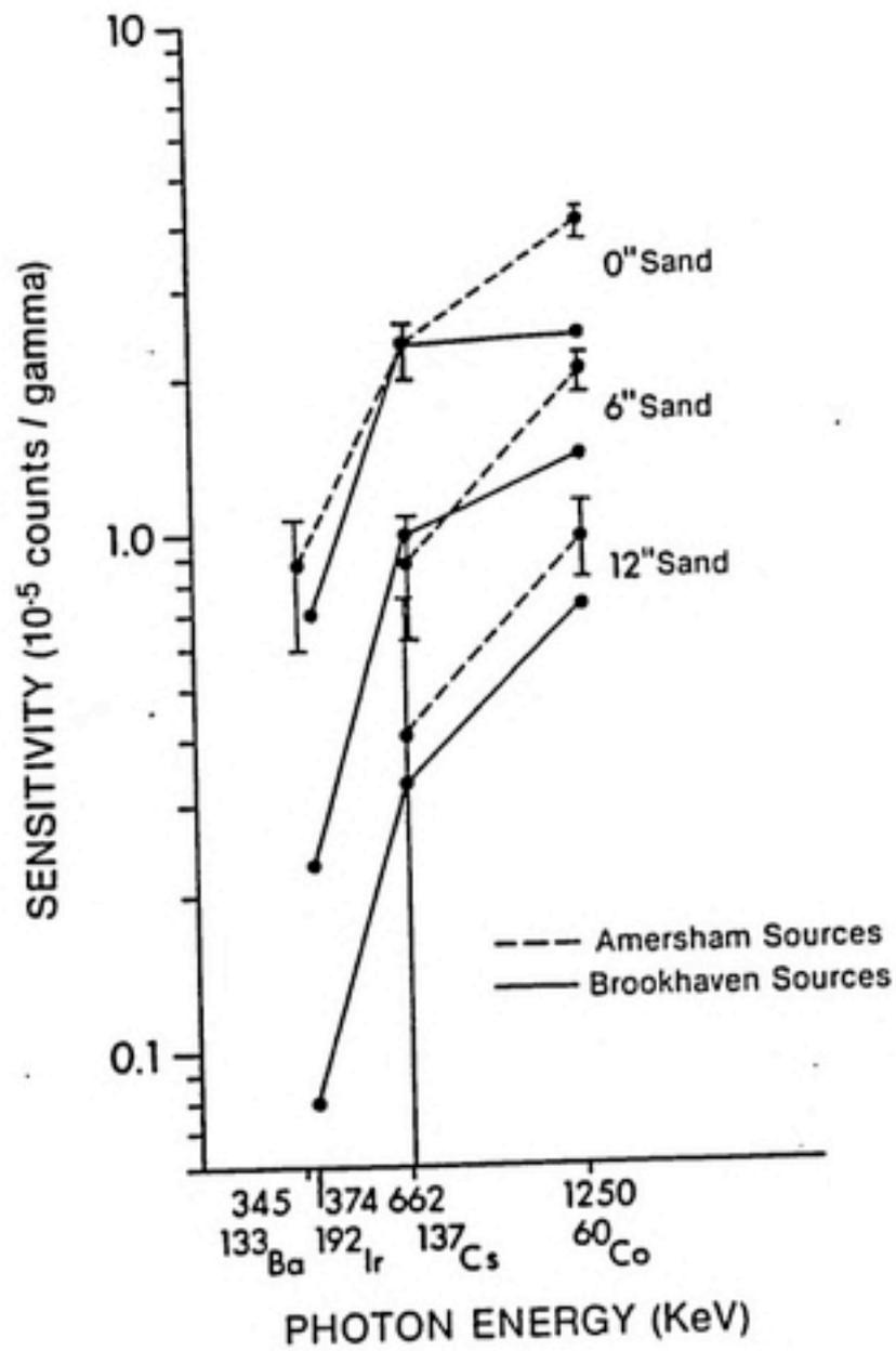
Figure 13. Comparison of Stationary-Vehicle Sensitivity
