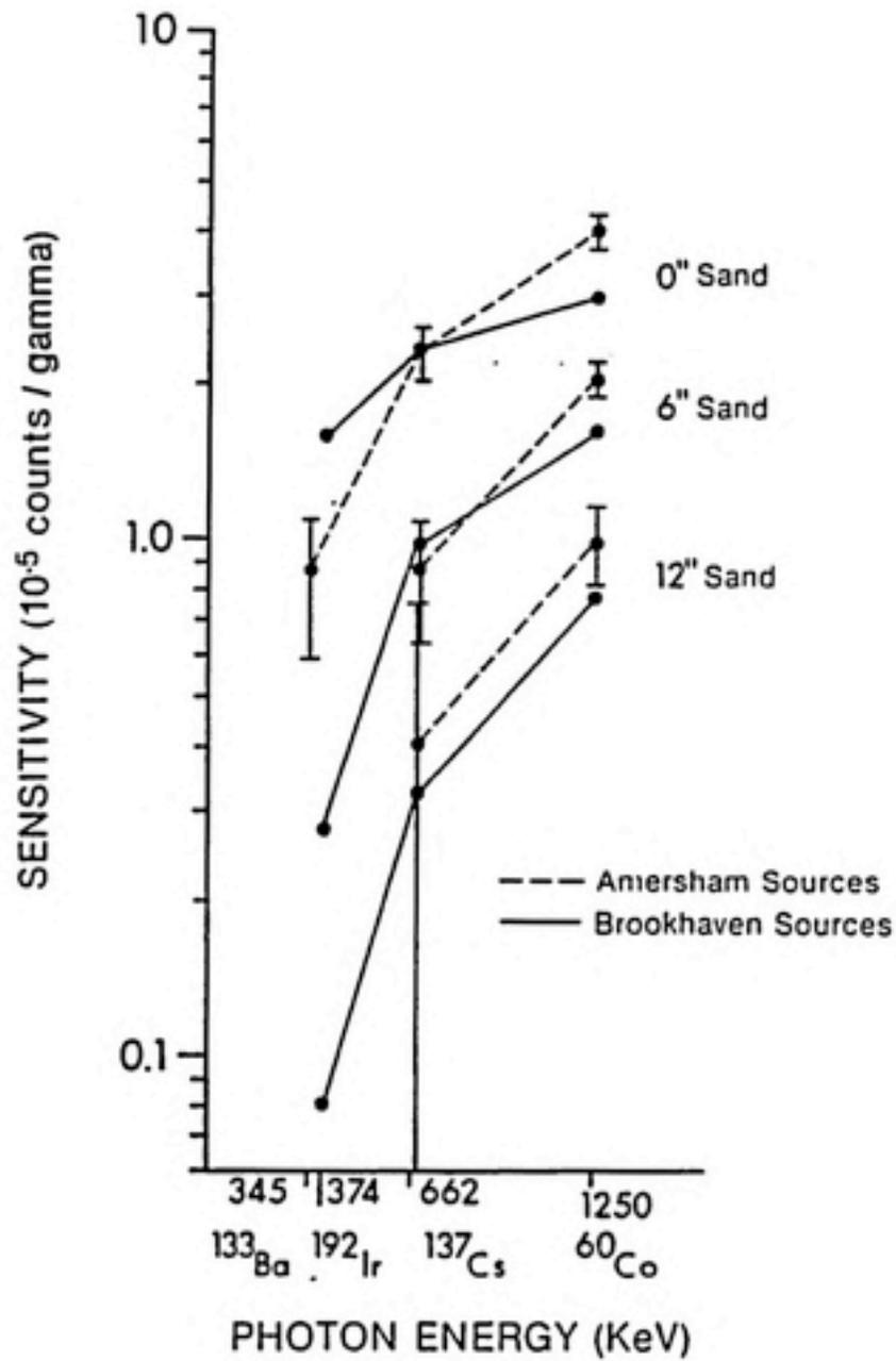
Figure 14. Comparison of Stationary-Vehicle Sensitivity, Amersham and Brookhaven Sources (Dead Time Corrected Values)
