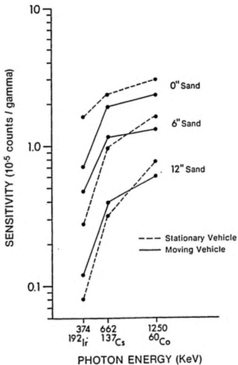
Figure 15. Comparison of Sensitivity for Brookhaven Sources (Dead Time Corrected Values) on Stationary and Moving Vehicle
