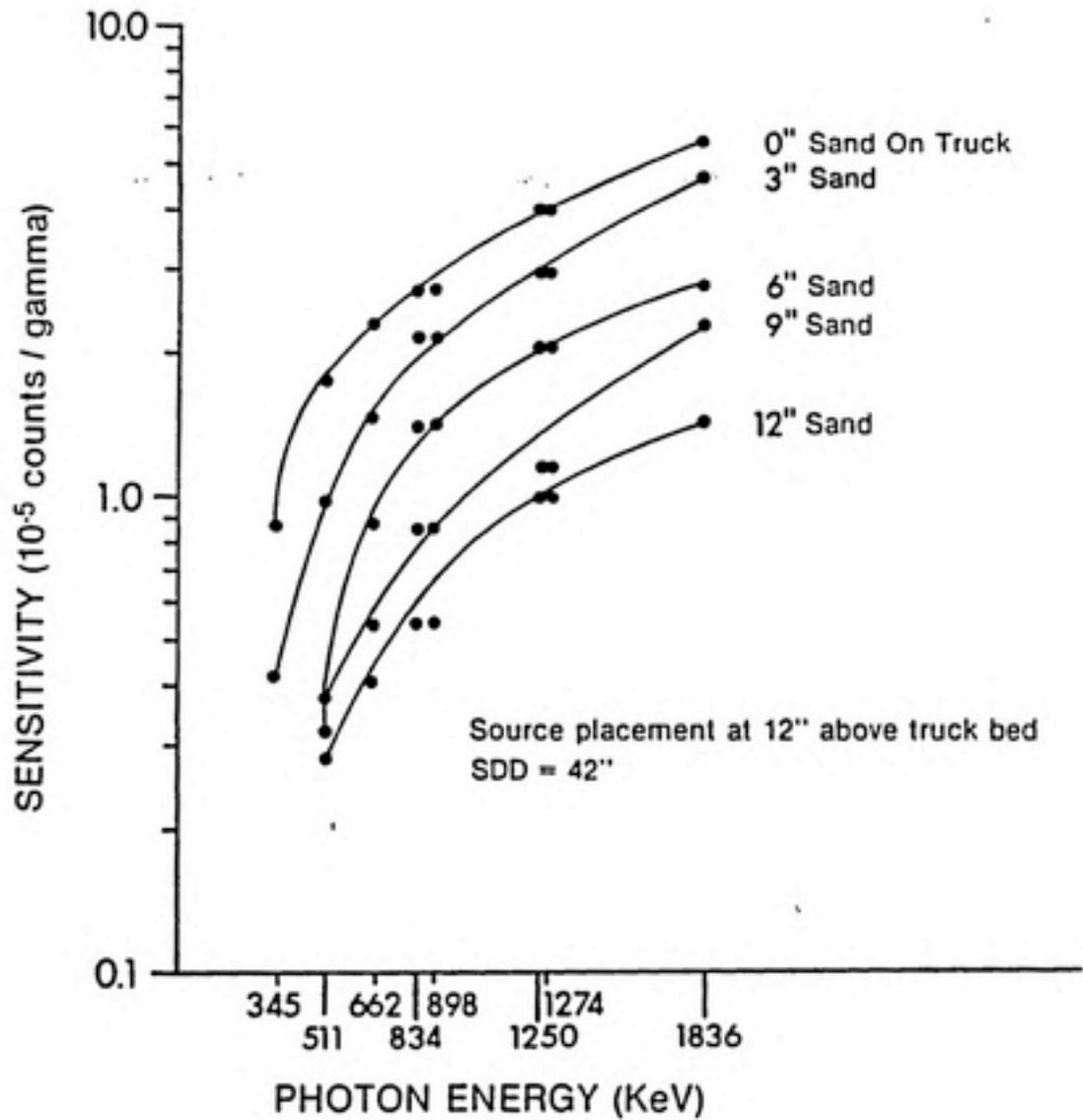
Figure 11. On-Vehicle Sensitivity Curves, Amersham Sources on Stationary Vehicle
