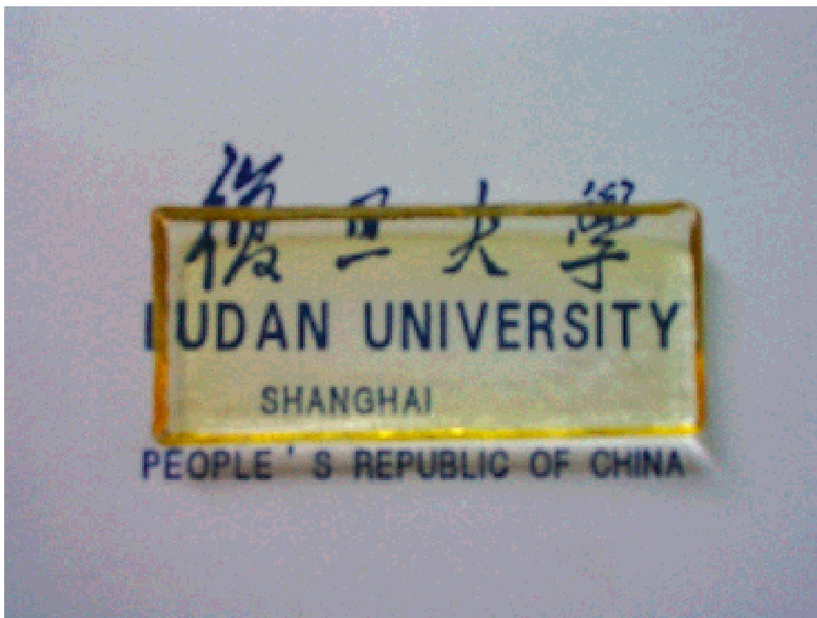
Figure 3.4: Photograph of an ordered transparent mesostructured block copolymer-silica monolith. Taken from (Yang et al., 2003)
