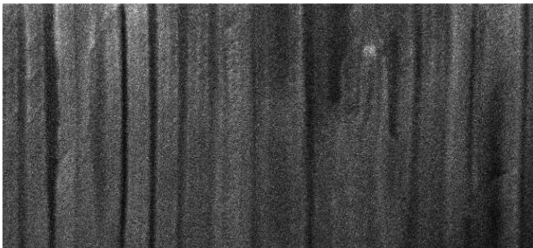
Figure A.1: Profile view of a 55 nm pore diameter Synkera AAO template broken in half to expose the pore structure.
