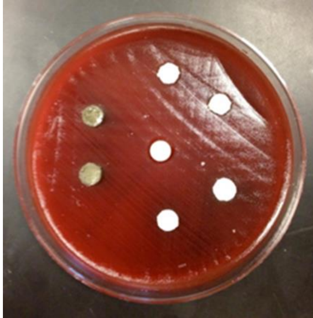
Figure 7 Photograph of the zones of inhibition in Enterococcus faecalis . In the dish, the upper right: GEMOSIL CHX , lower right: GEMOSIL, left: MTA, and center: Chlorhexidine.
