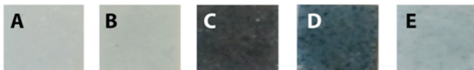
Figure 4.7. Hydrogen detection during reaction. A = Untreated polymer. B = Reaction, no light. C = H 2 -treated polymer. D = Reaction with light. E = Reaction with light, no catalyst.
