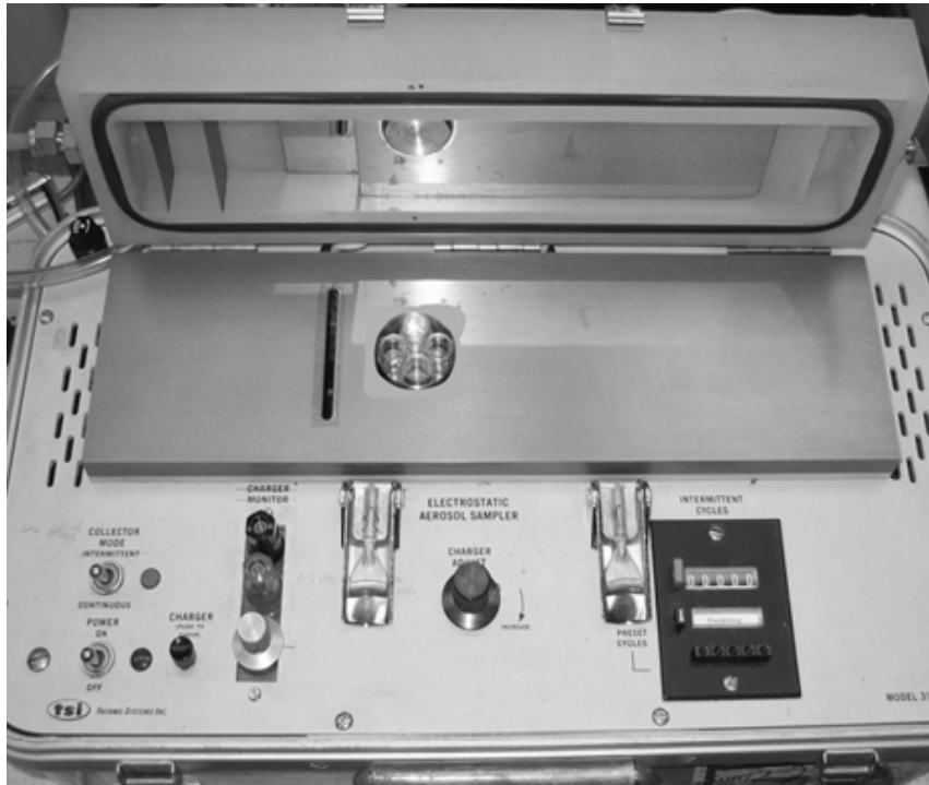
Figure 2-1. Top view image of the Electrostatic Aerosol in Vitro Exposure System (EAVES) holding the four Millicells
