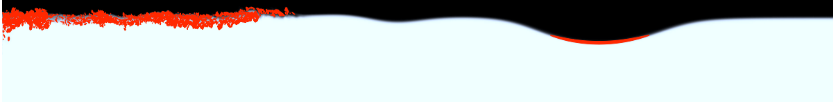
FIGURE 4.18. Density field at time t = 45 s, for a numerical experiment in which no shear instability has been observed. The amplitude ( a/h_1 ) of the solitary wave constructed from the second time series is 1.23 (wave IV in Figure 4.6). Regions in the flow field with Ri < 1/4 are marked with red.
