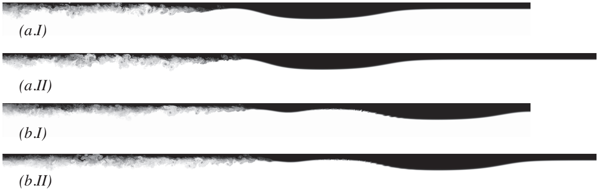
FIGURE 4.21. Density plots for numerical experiments with the same initial condition L_{gate} = 100 cm, h_{gate} = 53.21 cm. (a) Density plots at t = 39.45 s (a.I) tank of length 1232 cm, (a.II) tank of length 1386 cm (b) Density plots at t = 53.3 s (b.I) tank of length 1232 cm, (b.II) tank of length 1386 cm.
