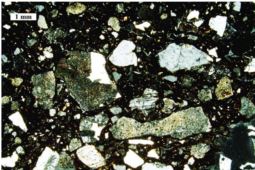
Figure 6.7. Highly-altered quartz + feldspar rock fragments (left of center) and feldspar mineral fragments (bottom center) in sample JMH048 (cross-polarized light). The feldspar in the rock and mineral fragments displays fine-grained sericite alteration. Also note the unaltered blocky plagioclase fragment (polysynthetic twinning; center).
