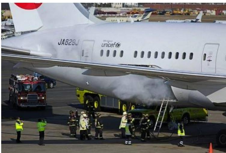
Figure 1.4 Japan Airlines Boeing 787 Dreamliner at Boston Logan Airport with smoke from battery fire.<sup>14</sup>
