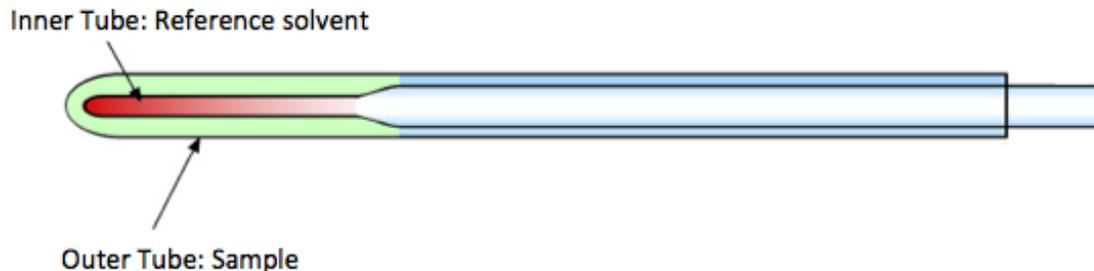
Figure 5.1 Schematic of NMR sample set up using a coaxial insert.<sup>6</sup>
