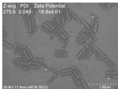
Figure 3.1 SEM and DLS of 80x320nm Hydrogel particles conjugated with DOTA
