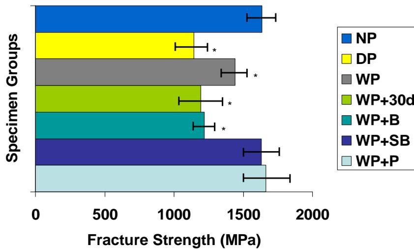
Figure 4.1 Flexure strength of Y-TZP bars reported in Table 4.1.
