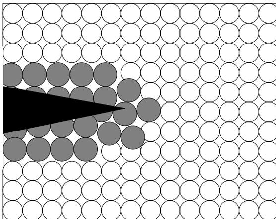
Figure 2.3 Schematic representation of effect of internal compression discouraging crack propagation. (After Jeff Thompson)
