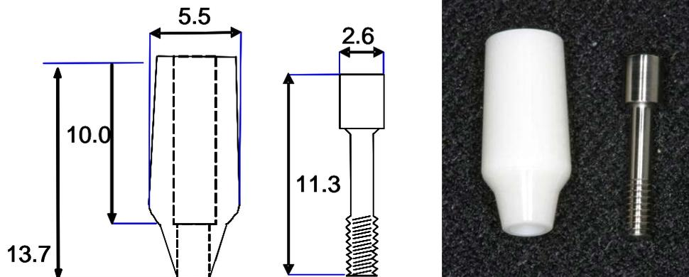
Figure 3.3 Abutment and abutment screw specifications and image
