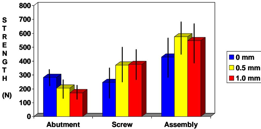
Figure 4.5 Peak load for each portion of the load-deformation curve depicted above in Figure 4.4 for each assembly group.
