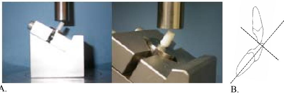
Figure 3.9 Assembly testing regime. A. Testing apparatus for loading assemblies containing prepared abutments. B. Schematic of forces applied.
