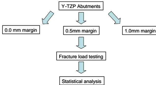
Figure 3.2 Flowchart of ZrO<sub>2</sub> abutment preparation and testing.
