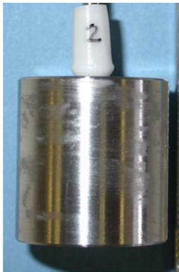
Figure 3.8 Abutment assembly fixed within implant analog with Field's metal.
