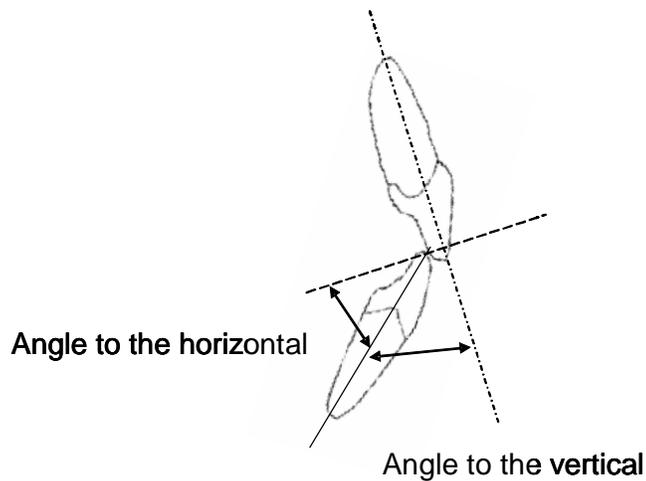
Figure 2.4 Horizontal and vertical reference lines for reporting loading angles.
