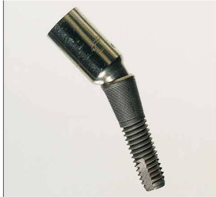
(a) Two piece, deformation at internal hex.
