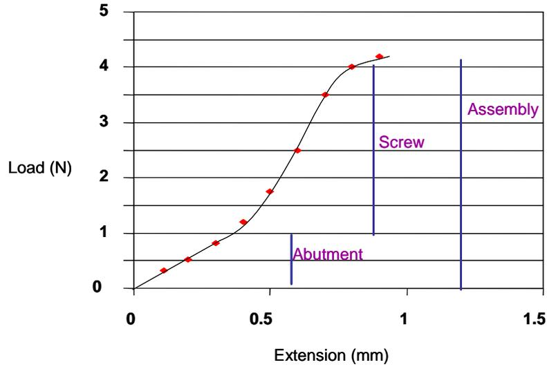
Figure 4.4 Schematic representative of typical load-deformation curve. (Vertical lines indicate the different assembly parts seemingly associated with the major deformations.)
