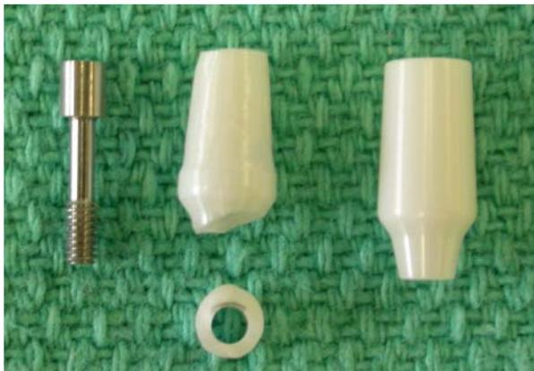
Figure 4.3 Indication where typical abutment fracture occurred.
