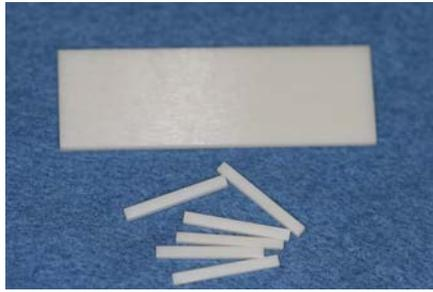
Figure 3.5 Image of Y-TZP plates and cut bars.
