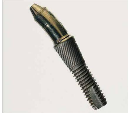
(b) One piece, deformation at body of abutment.
