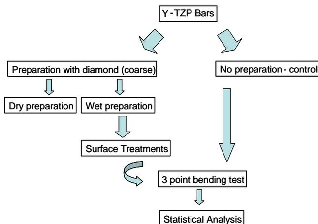
Figure 3.1 Flowchart of methods for Y-TZP preparation and testing.
