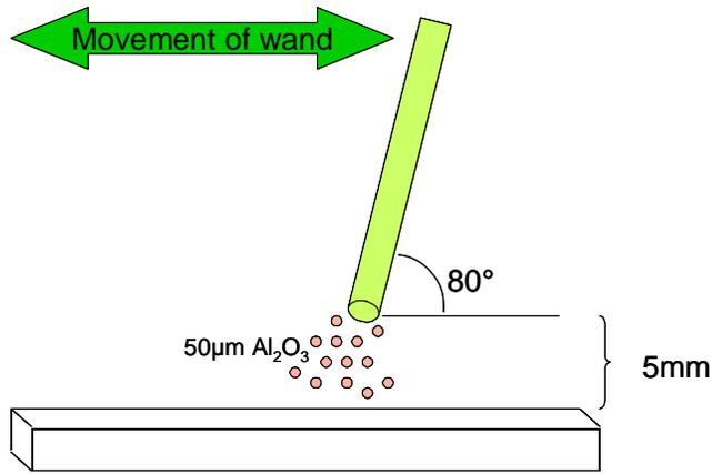
Figure 3.6 Diagram of sandblasting method.
