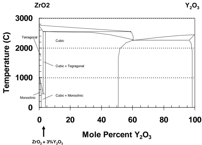
Figure 2.2 Phase diagram for ZrO<sub>2</sub> – Y<sub>2</sub>O<sub>3</sub>. (After Levin *et al.*, 1979)
