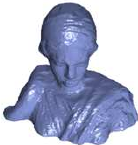
Figure 1.2: A 3D model of a statue reconstructed from 36 images. The object was placed on a turn-table and imaged under fairly controlled conditions.
