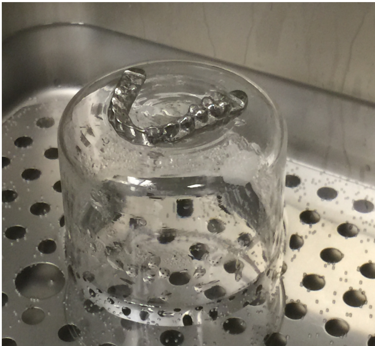
Figure 21. A reference appliance in the water bath to bring its temperature close to the oral temperature.
