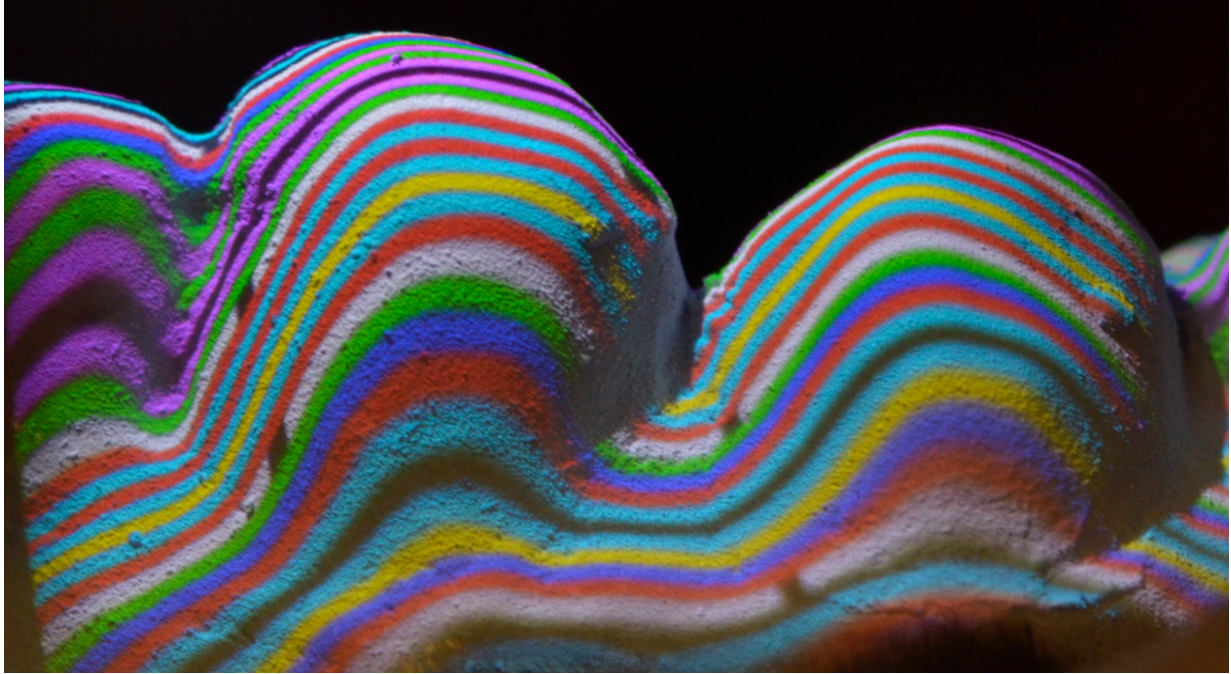
Figure 2. Omnicam stripe pattern.
