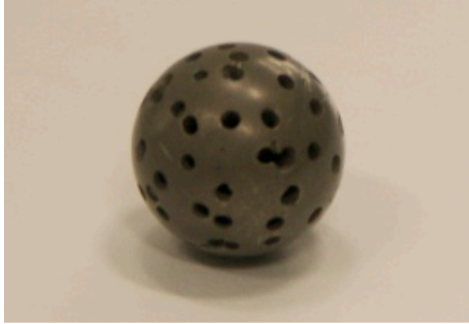
Figure 5.6: Picture of a plastic drilled sphere used in this sections experiments with radius A = 0.635 cm, mass m_s = 0.8986 g, and porosity P = 0.38 .
