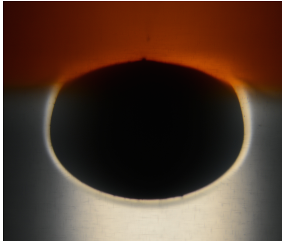
Figure 8.7: Experimental picture showing the thin shell around the sphere for entrainment dominated regimes.
