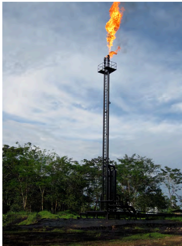
Figure 10 A flare tower in the Amazon visible on the ground surrounding the flare is an area covered in crude oil particles that have coated the surrounding vegetation. Photo by author, 2013.
