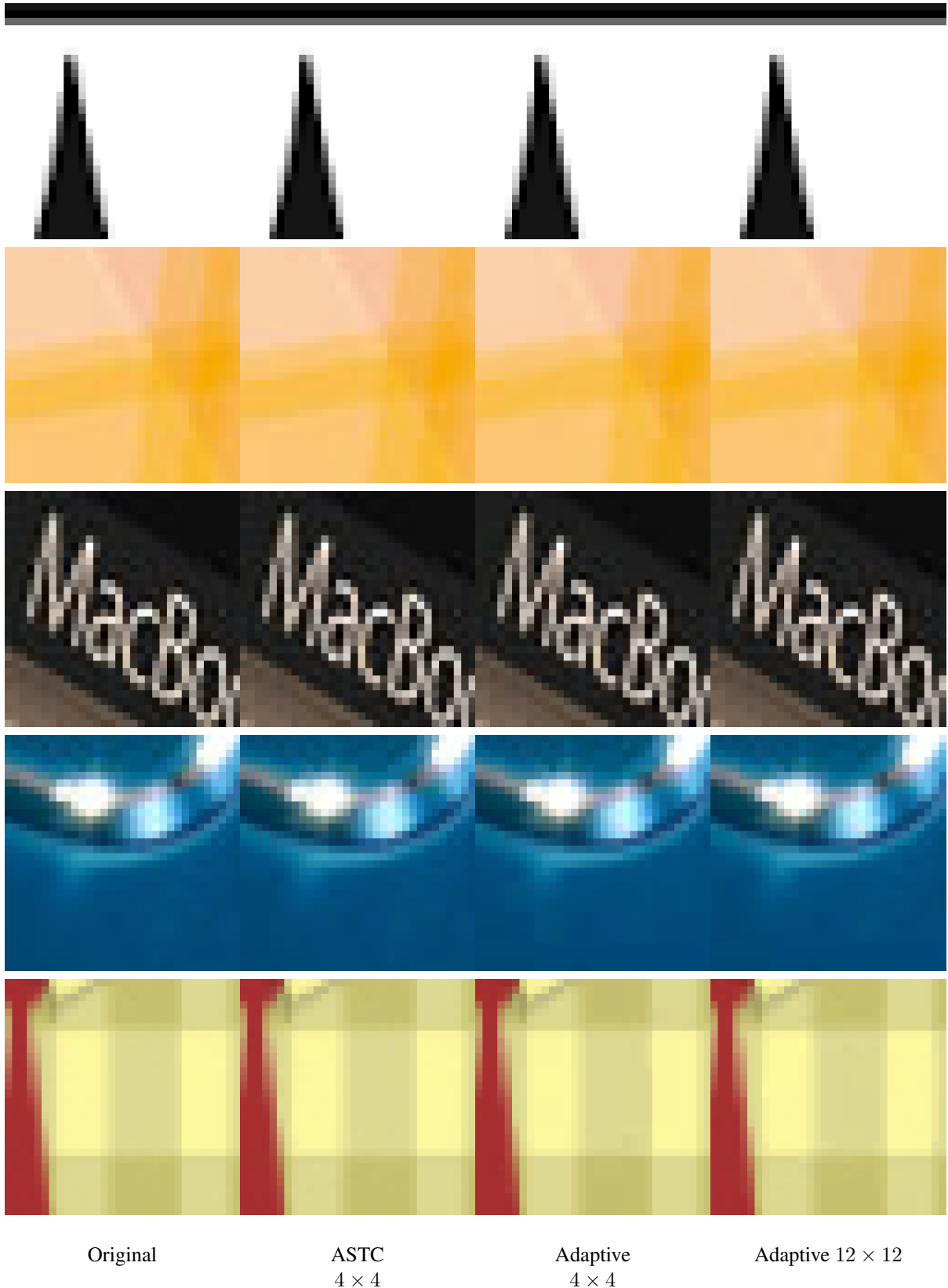
Figure 5.11: A comparison of the compression artifacts generated by each algorithm. We compare our method against Adaptive Scalable Texture Compression (Nystad et al., 2012). As in Figure 5.10, our adaptive compression schemes require the error for each grayscale block to be within \|\Delta B\|_\infty < 4 and each color block to be within \|\Delta B\|_\infty < 8 .
