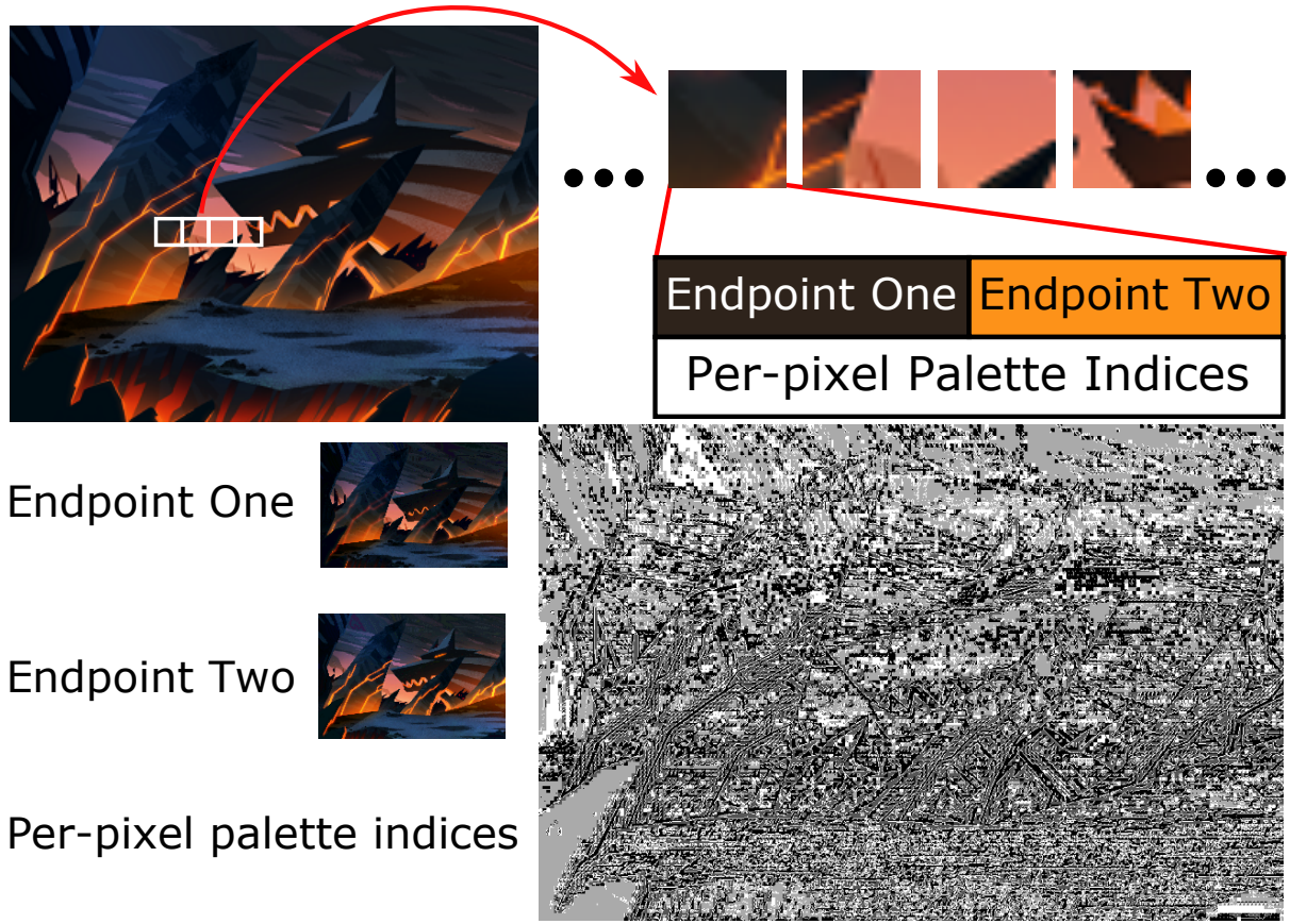
Figure 6.1: The constituent parts of a compressed texture. Each endpoint compressed texture represents a sequence of equally sized blocks. Each block contains a fixed number of bits containing two endpoint colors that generate a palette and per-pixel index data. Here we show the endpoints separated into individual images and visualize the per-pixel indices. We re-encode the indices using VQ-style dictionary compression and transform the endpoint images using a wavelet transform prior to encoding the final texture using an entropy encoder.
