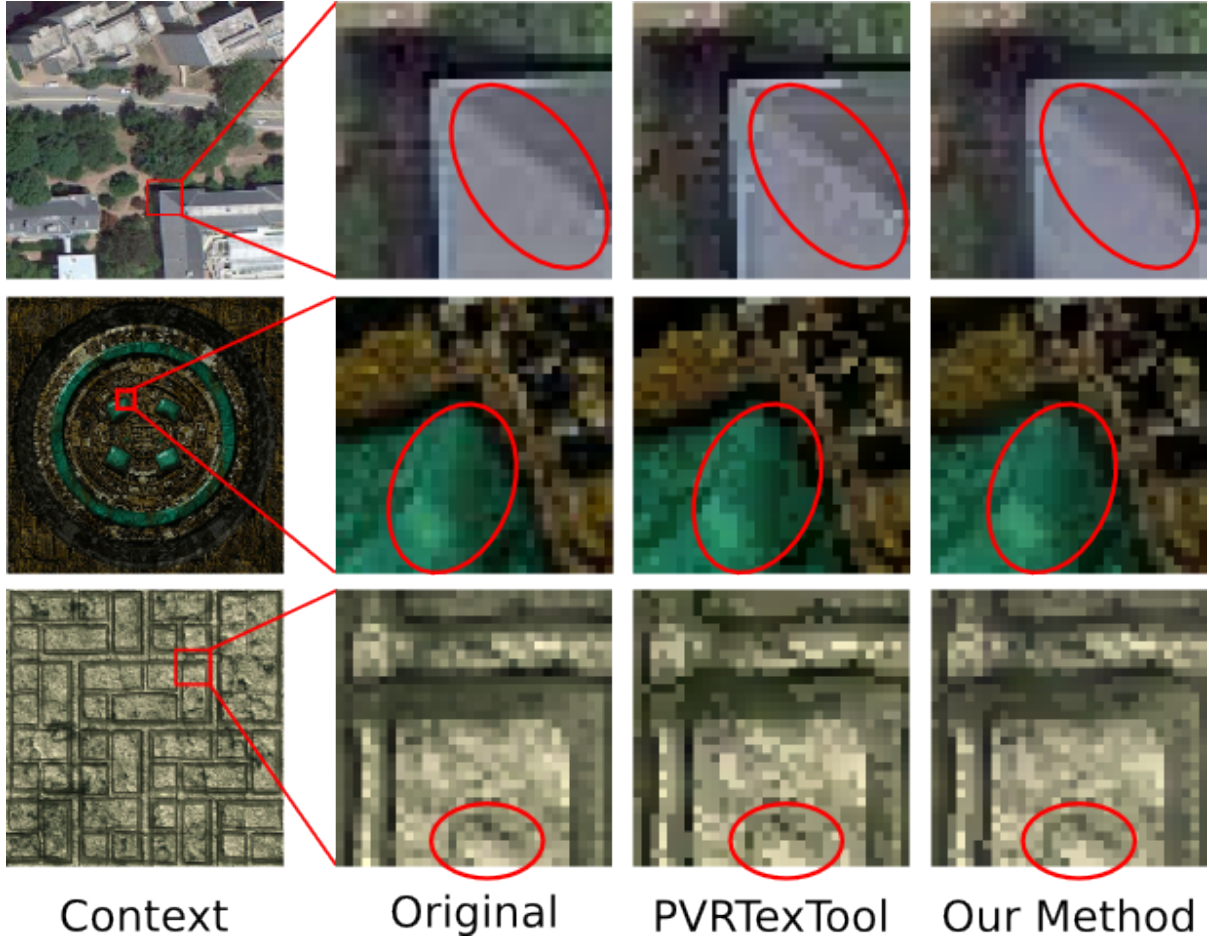
Figure 4.9: Investigation of areas with high detail in some common mobile graphics images. We notice that the texture compressed using intensity dilation maintains the smoothness of many image features, while the original PCA based approach leaves blocky streaks. Images courtesy of Google Maps, Simon Fenney, and http://www.spiralgraphics.biz/ .
