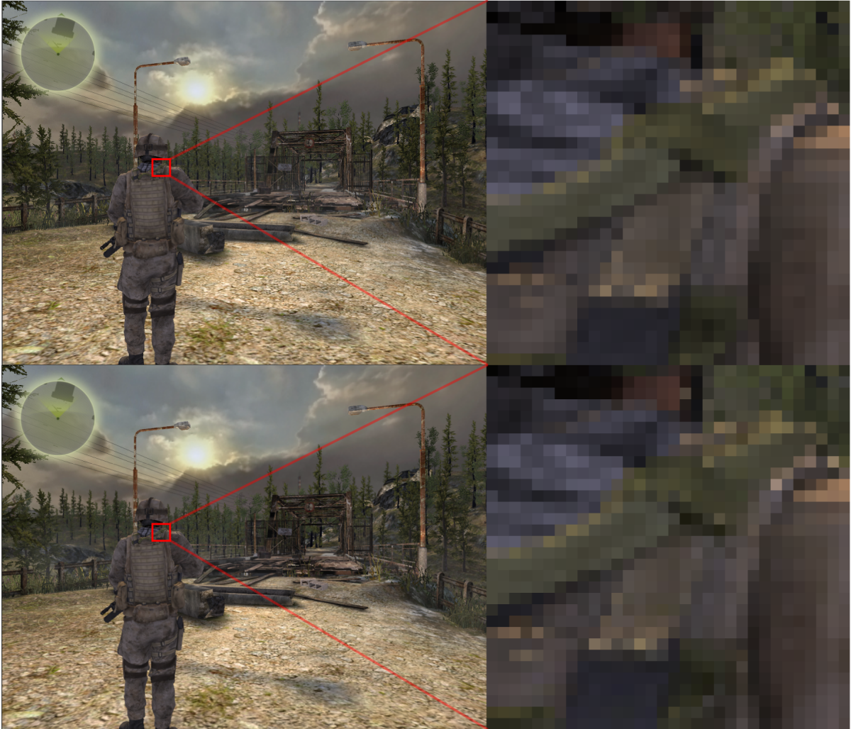
Figure 4.1: The Bootcamp demo from Unity3D 2 using uncompressed textures (top) and using textures compressed with FasTC-64 (bottom). The visual quality of the scene is only slightly altered and no visible artifacts appear. The scene uses 156 textures which were compressed in a total of 8.75 minutes by our method. The same textures are compressed by the BC7 Compressor in the NVIDIA Texture Tools in a total of 13.27 hours.
