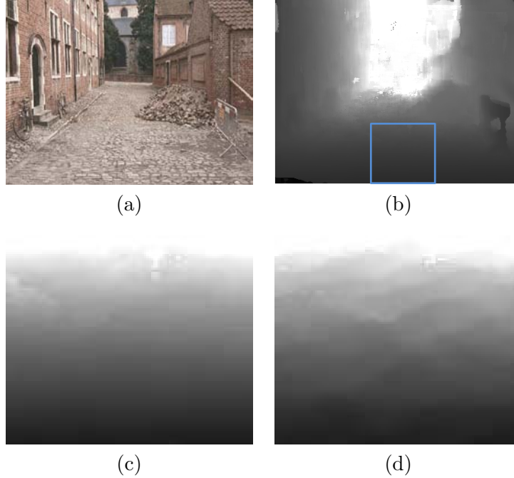
Figure 4.6: (a) Original image. (b) Depthmap computed using our multi-sweep method. Close-ups are shown for the marked area. (c) Close-up of the multi-sweep depthmap. (d) Close-up of the fronto-parallel sweep depthmap. Notice the staircase artifacts.
