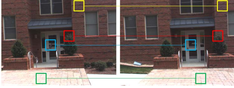
Figure 2.6: Difficulties with matching. (Red) The matching window overlaps a depth discontinuity. (Green) The matching window is affected by perspective distortion. (Blue) The matching window contains a reflection. (Yellow) A good match is obtained.
