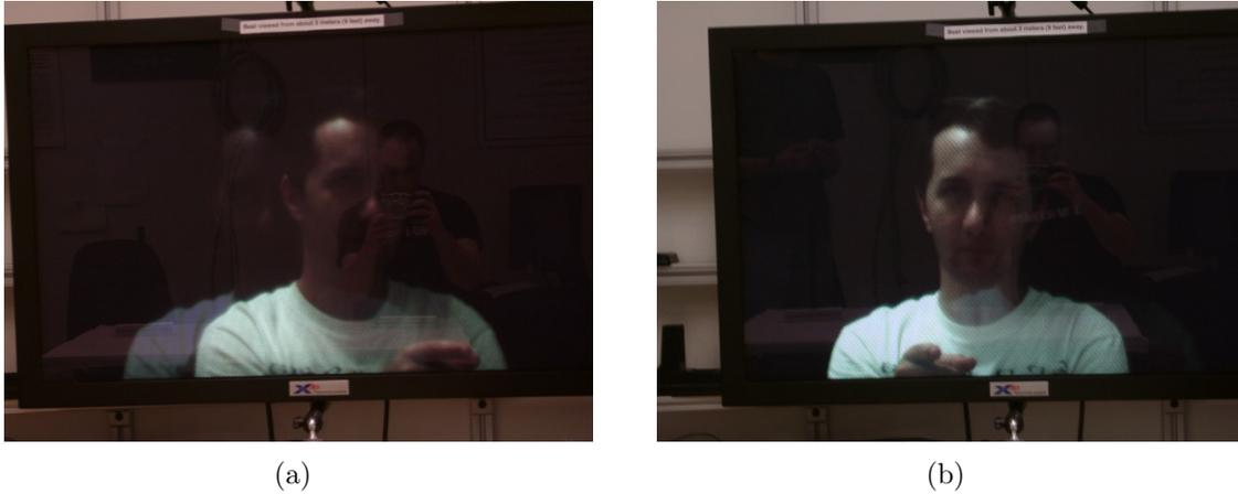
Figure 5.4: Newsight 40” autostereoscopic 8 view display showing two live views. Notice the ghosting between views; imagery from one view is partially seen in the other.
