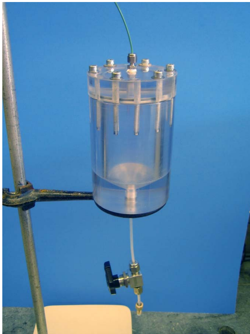
Figure 2-7: Polycarbonate slurry reservoir used to pack anion exchange columns. The green PEEK tubing at the top of the reservoir connects to a HPLC pump, which generates the flow used to pack the column. The metal valve at the bottom controls the flow of slurry into the column to be packed, which is connected using the tan PEEK fitting at the bottom of the image.
