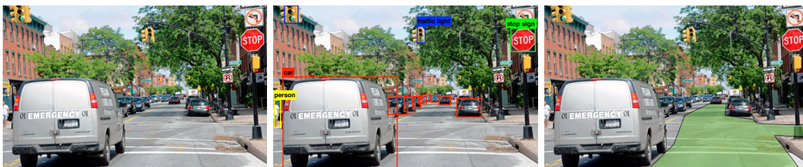
Figure 1.1: This dissertation studies the problem of object detection and semantic segmentation . Object detection is to know the location (e.g. bounding box) of each object; and semantic segmentation is to know what each pixel is (e.g. drivable path) in an image.
