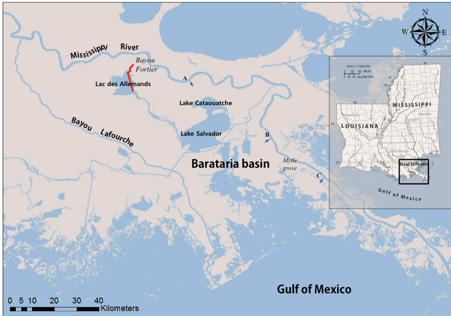
Figure 4. The study area is in Barataria Basin in the Mississippi River Delta, ^{222}\text{Rn} survey routes (a red line) and the Mississippi River diversion locations (A, B, and C blue arrows) are shown. Note that a red arrow indicates ^{222}\text{Rn} survey direction from mouth of the lake to the upper Bayou Fortier. *Mississippi River diversions - A: Davis pond; B: Naomi; C: West Pointe a la Hache
