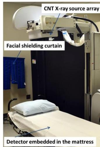
Figure 2.8 The s-DCT prototype installed at the Cystic Fibrosis and Pulmonary Diseases Research and Treatment Center, at UNC Marsico Lung Institute for clinical trials
