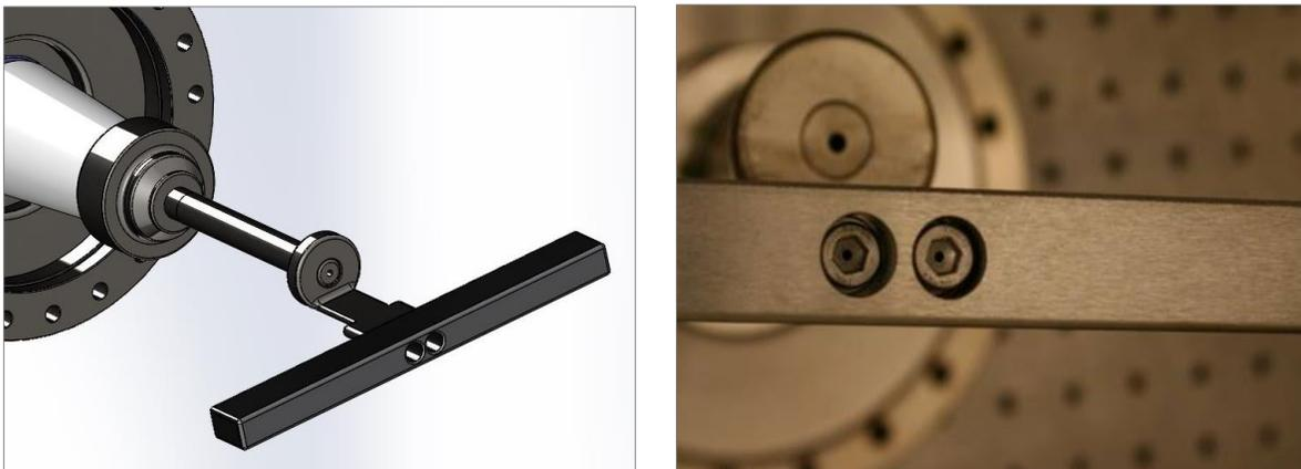
Figure 3.25 SolidWorks drawing and a photograph (bottom view) of the anode assembly highlighting the two setscrews at the bottom of the anode.
