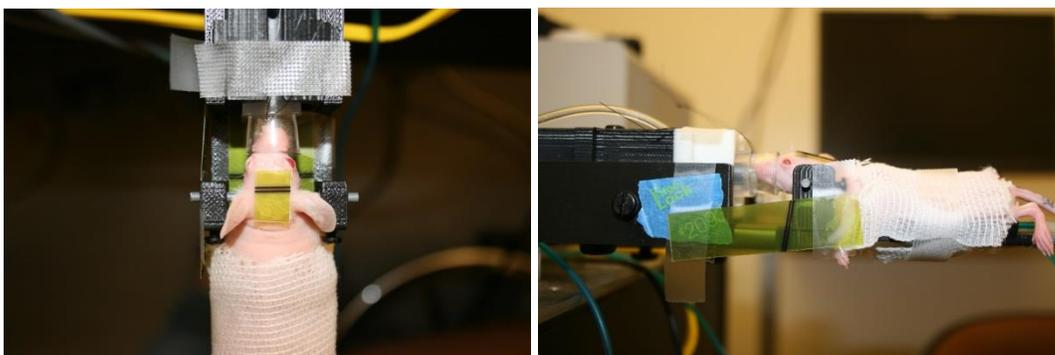
Figure 5.6 Pictures of the recovering animal on the mouse holders. As shown here, Gafchromic films were placed at the beam entrance, exit, as well as on the side of the mouse bed, to verify the delivered radiation dose and beam patterns.
