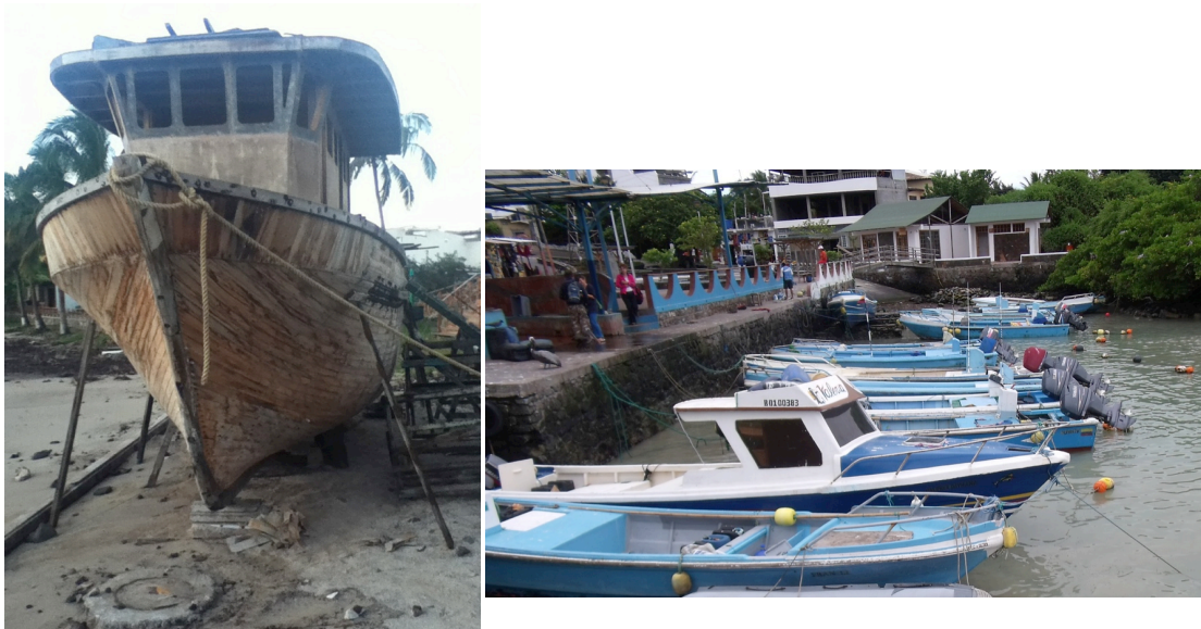
Figure 2.2. Various vessel types in the Galápagos fishing fleet. A larger wooden bote on the left in construction. Botes are given a coat of paint before going to sea. A line of fibras and pangas on the right, which are similar in shape but differ in material and length. The boat with a cabin in the foreground is a fibra . Photos by author.
