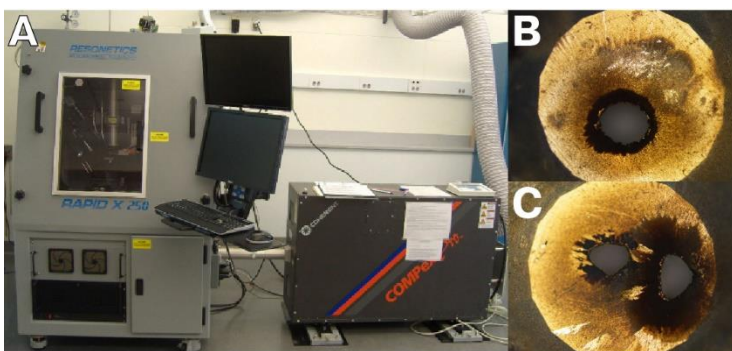
Figure 2.23 | Laser ablation for hole burning. (A) Laser ablation instrument in CHANL. (B, C) examples of holes burned using a laser. High charring and asymmetry are characteristic of all holes burned.
