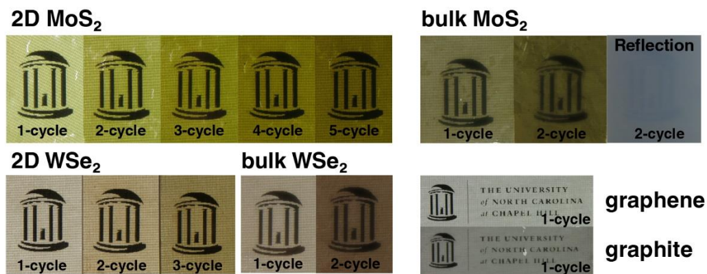
Figure 2.9 | Transparent films of 2D materials via LB trough deposition. Scale: the “Old Well” = 1 cm wide. All 2D materials were prepared via method 1 protocol of section 2.2.
