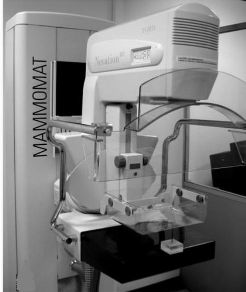
Figure 1.4 Mammomat – the prototype tomosynthesis system from Siemens [15].
