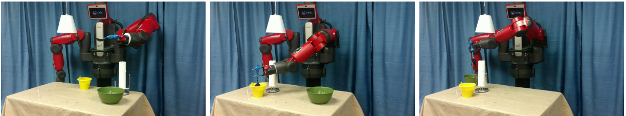
Figure 3.1: As the Baxter robot performs the learned task of transferring powder from the yellow bucket to the green bowl using the blue spoon, a person moves the green bowl. Our method automatically replans in a closed-loop manner, enabling the robot to avoid obstacles and perform the learned task even when task-relevant objects or obstacles are moved mid-task.
