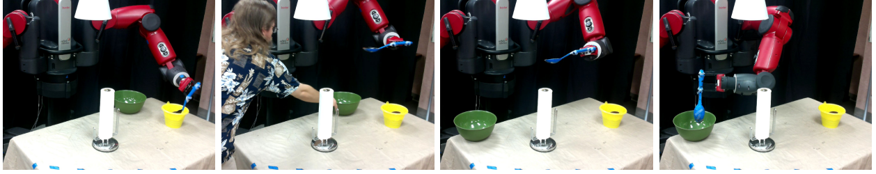
Figure 4.3: The Baxter robot performing the powder transfer task with the spoon being used as a tool in blue, the source container in yellow, and the destination container in green. Both the lamp and paper towel obstacles are white.
