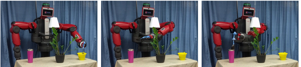
Figure 5.13: Using the method of Bowen et al. [16] we learned a task wherein the Baxter robot scooped powder from the yellow container and transferred it into the magenta one without spilling while avoiding obstacles in the environment.
