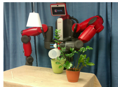
(c) Rethink Robotics Baxter robot autonomously performing a liquid pouring task.
