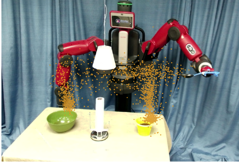
Figure 3.4: End-effector positions of sampled configurations (shown in blue) from the biased distribution for the task of scooping powder from the yellow bucket into the green bowl. The distribution is dependent on the landmark positions. Sampling configurations in useful places enables us to build higher quality roadmaps with fewer samples, which facilitates faster motion planning.
