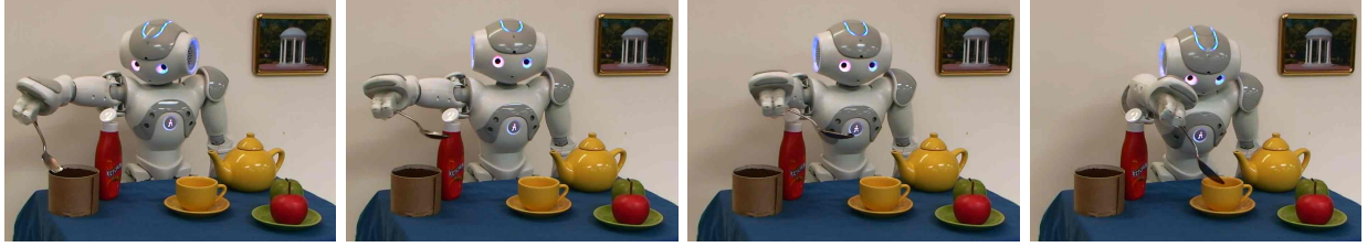
Figure 2.7: Execution of DGMP for the powder transfer task. The robot successfully keeps the spoon level while avoiding obstacles not seen in the demonstrations.
