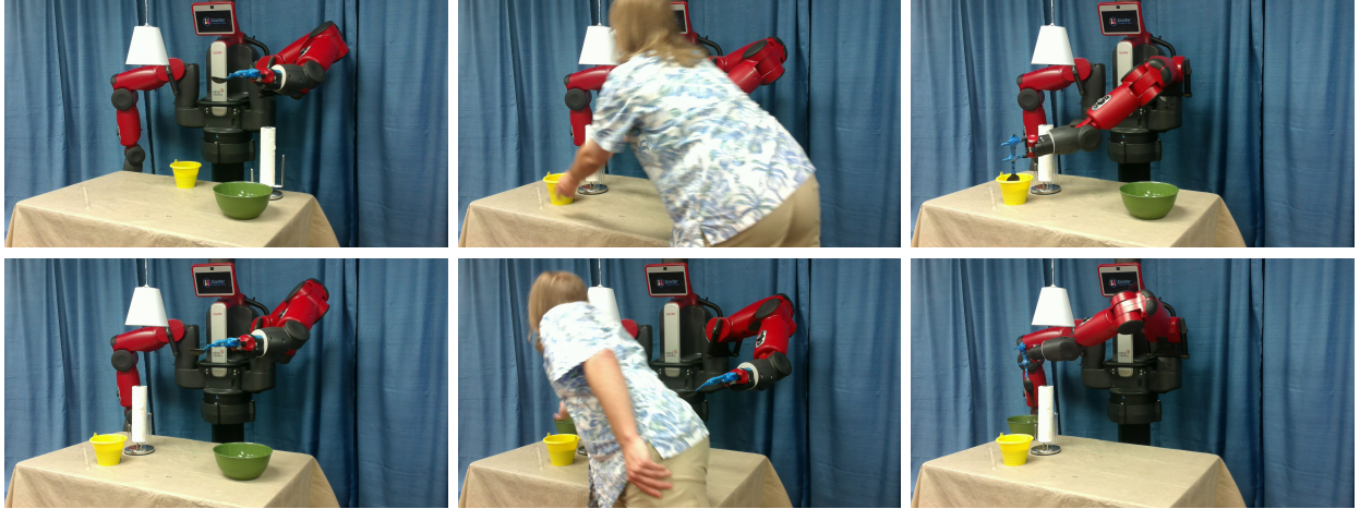
Figure 3.8: Example execution for the powder transfer task, from a bucket (yellow) to a bowl (green).
