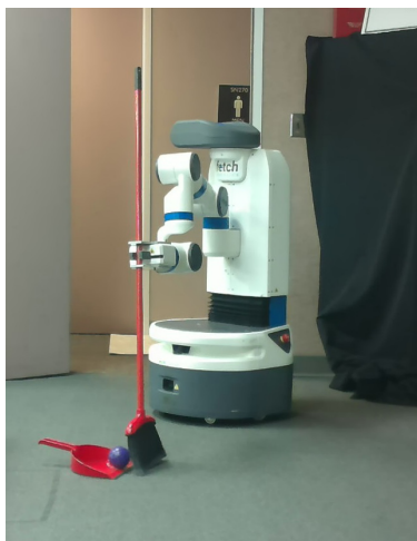
(b) Fetch mobile manipulator robot autonomously performing a sweeping task.
