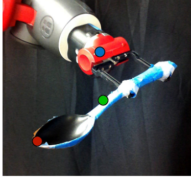
Figure 4.4: A spoon being used as a tool in the powder transfer task with an arbitrary landmark at the robot’s gripper marked in blue, the hand-picked landmark at the tip marked in red, and the tool virtual landmark learned by our method marked in green.
