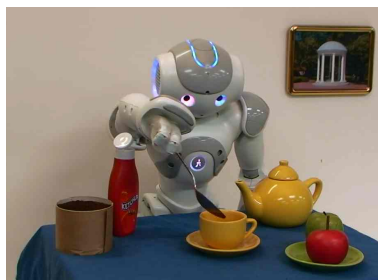
(a) Aldebaran Nao robot autonomously performing a powder transfer task.
