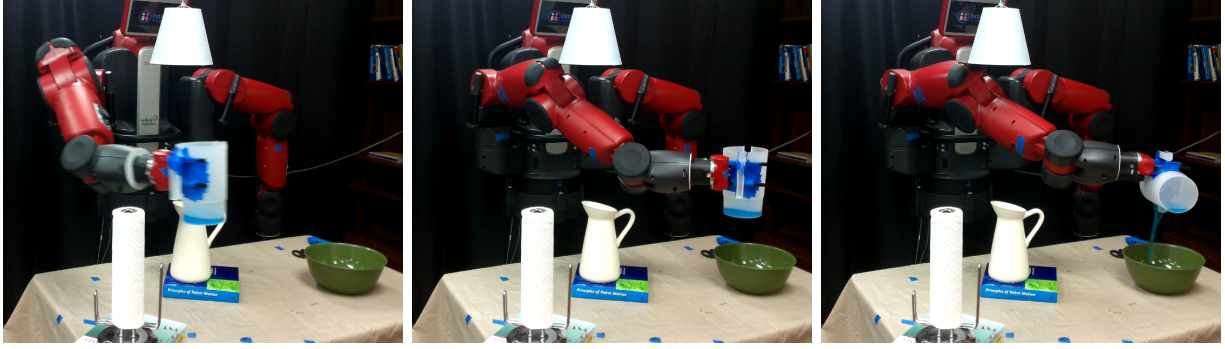
Figure 4.5: Baxter robot performing the liquid pouring task with the pitcher (being used as a tool) with blue liquid and the green bowl. The lamp, vase, and paper towel obstacles are white.
