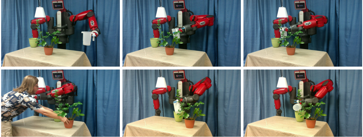
Figure 3.9: Example execution for the liquid pouring task, from a pitcher into a pot (green).
