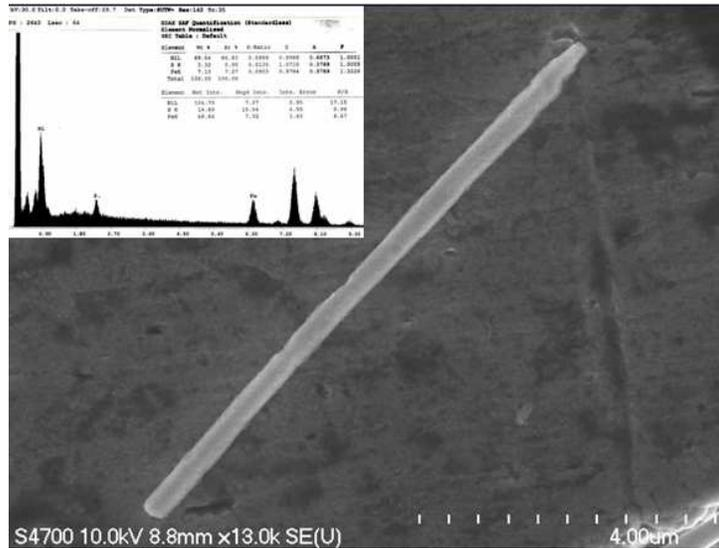
**Figure 2.6**, SEM image of a released Ni:Fe nanowire. The radial dimension is around 200 nm and the length is about 9 μm. The insert is the EDAX measurement of an etched Ni:Fe plated AAO membrane.
