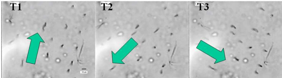
**Figure 4.10**, An array of magnetic nanowires rooted inside a supporting PDMS layer, beating with a triangular orbit inside a flow channel. Snapshots were taken by a built-in CCD camera in 3DFM *Betty* 1. The time sequence was pre-set so that a triangular orbit beating with 2/3 Hz could be performed. Each short black rod feature is a tilted nanowire projected in 2D. Arrows shown here are the schematic actuating magnetic field directions which are projected to the image plane.
