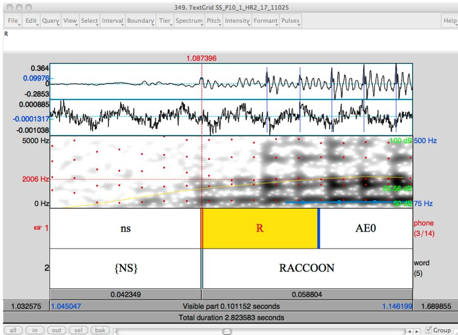
I moved the boundary to where the waveform starts looking more like the oscillations to the right as opposed to the left. The boundary also marks the position of the appearance of a second formant.
