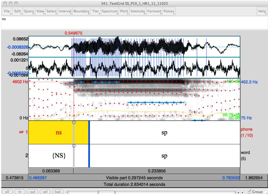
The algorithm has incorrectly identified its onset. I moved the boundary to the onset of the 4602 frequency band.
