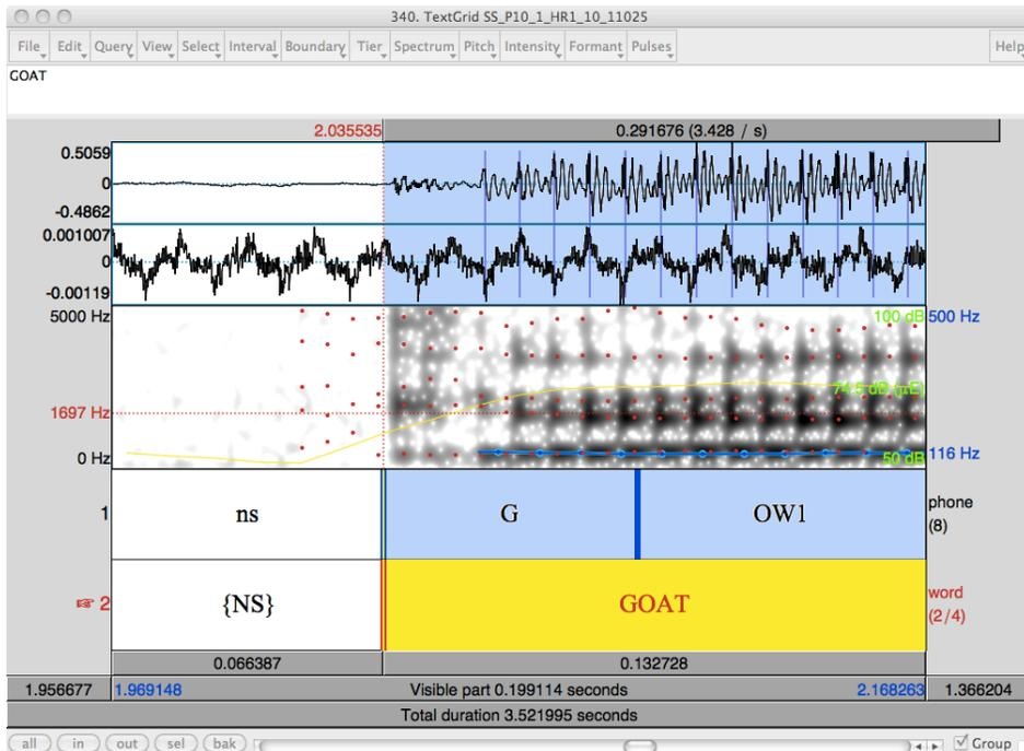
For fricatives such as s,z,f,v,th, and affricates such as ts,tz the onset is marked by the appearance of a band of higher frequency. In the following screen shot I have zoomed into the onset of the word snail. The algorithm has again marked the onset of s earlier than it should have.
