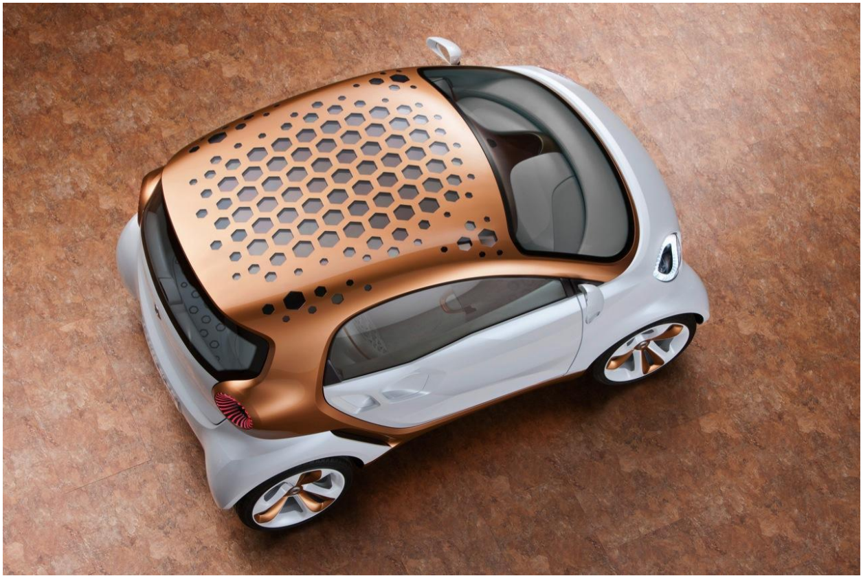
Fig. 19. Smart Forvision Conceptual Design by BASF and Daimler [23]. This image displays the conceptual design for a car utilizing transparent organic solar cells in the roof to improve the vehicle's energy efficiency.
