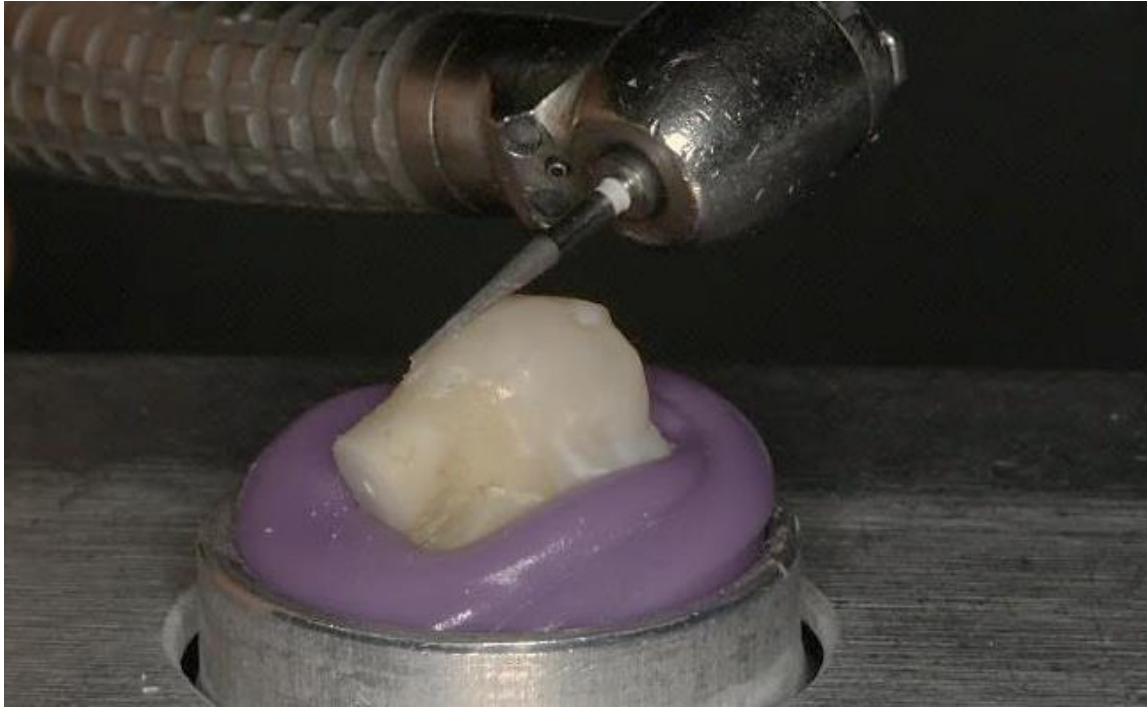
Figure 4. Finishing procedure using pressure device at approximately 0.15 N.
