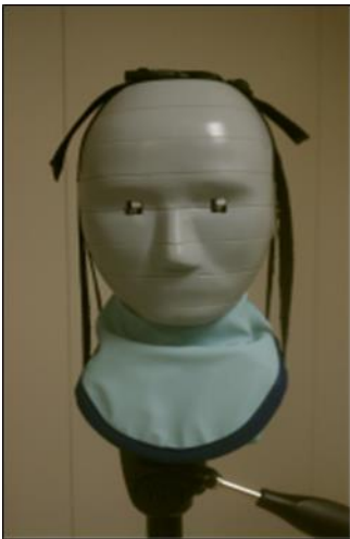
Figure 3.7: Child Tissue-Equivalent Phantom (w/Thyroid collar) (ATOMmax Model 706 HN, CIRS Inc., Norfolk, VA)
