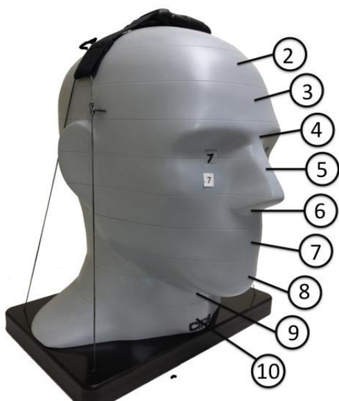
Figure 3.4: Average Adult Tissue-Equivalent Phantom (ATOMmax Model 711HN - CIRS Inc, Norfolk, VA)
