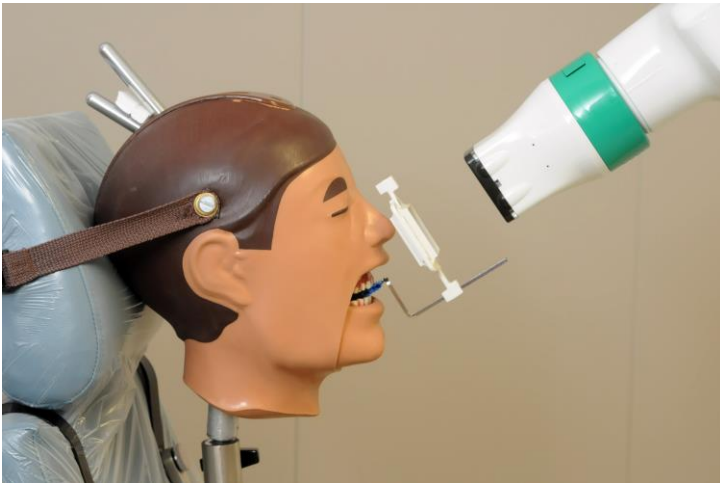
Figure 3.10: Test Collimator Beam Alignment Ring
