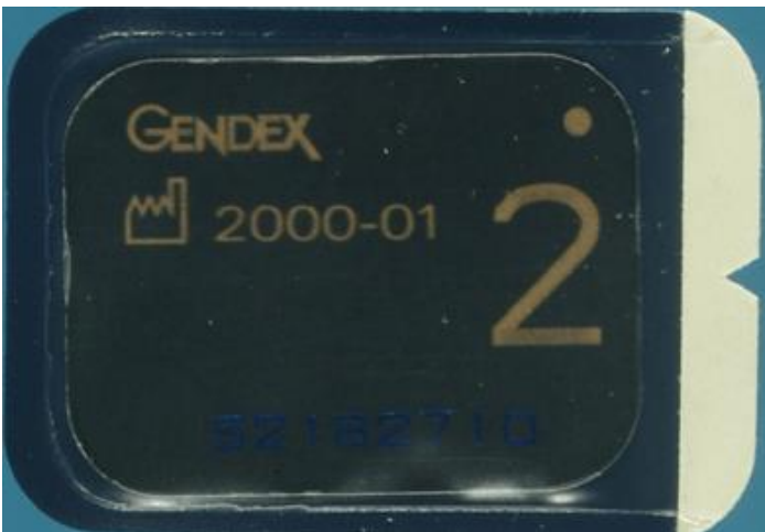
Figure 3.11: DenOptix® Photostimulable Phosphor Plate (PSP) receptors (Size 2 example)
