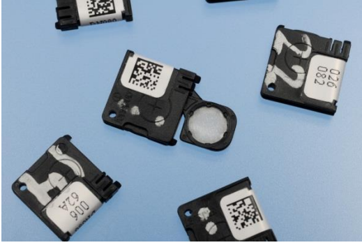
Figure 3.6: Nanodot OSL Dosimeters
