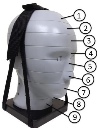
Figure 3.5: Child Tissue-Equivalent Phantom. (ATOMmax Model 706 HN, CIRS Inc., Norfolk, VA)
