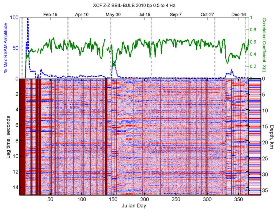
Figure 20. North flank crossing individual and 1 year stacked cross-correlation functions at station pair BBIL-BULB for 2010. Annotation is the same as for Figure 10.
