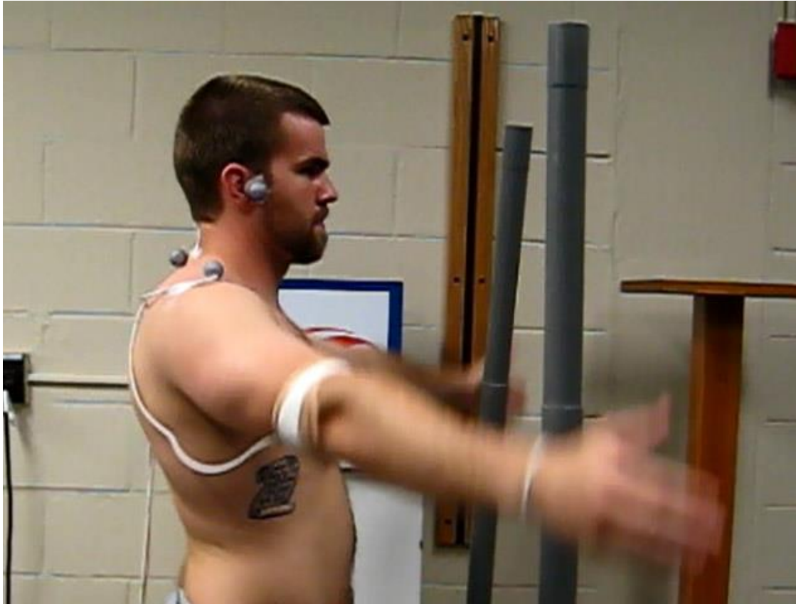
Figure 2 – Participant performing elevation task while equipped with electromagnetic motion tracking system
