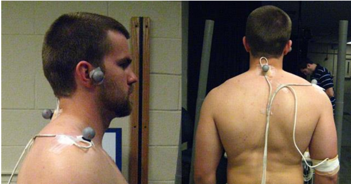
Figure 1 - Receiver and reflective marker placement for humerus, scapula, tragus and spinous process of C7
