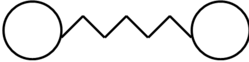
Figure 3. Toy model: The two atoms of a diatomic system interact with each other and this interaction is modeled as a one-dimensional spring that follows Hook's law, F = -kx , where k is the force constant and x is the displacement from the mean position.
