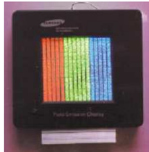
Figure 1.18: 4.5 in. CNT field emission display made using screen printing [27].
