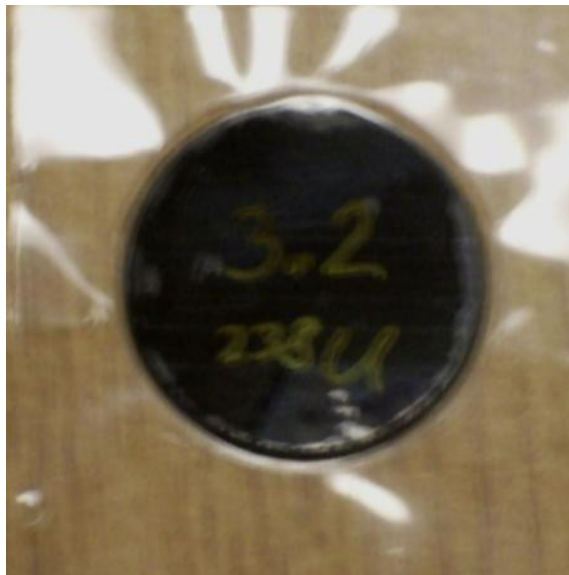
Figure 5.11: One slice of depleted uranium in its plastic sealant. Target diameter is 2.54 cm.
