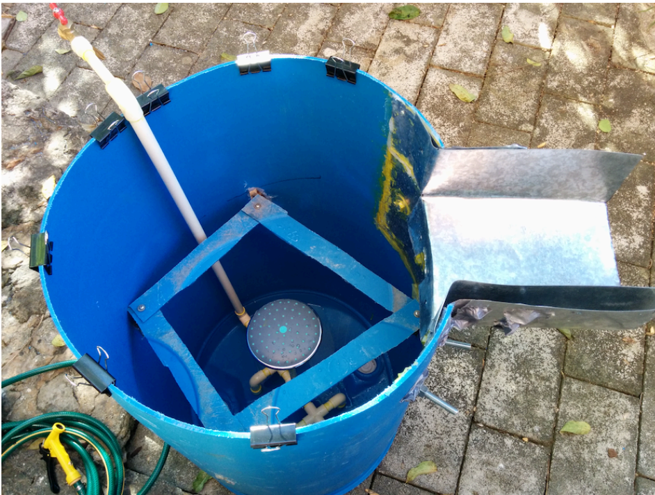
Figure 3.6. Photograph of the flotation machine, showing giraffe-like PVC pipe into which water would flow from a hose and exit through the showerhead toward the sample. There are two metal spouts on the right, one of which fits over a mosquito net inserted into the tank.
