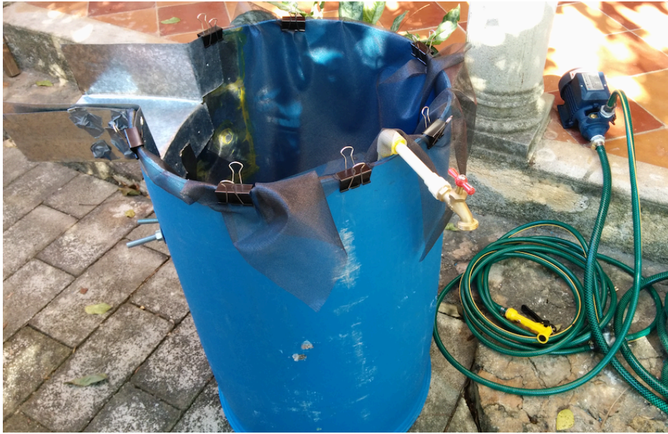
Figure 3.7. Flotation machine with mosquito net inserted. Below spout there will be a colander resting on a bucket, which holds the veil fabric used to collect the light fraction.
